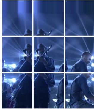
Figure 4. The results of 9 search regions. The region in the center is the area which methods based on Discriminative Correlation Filter (DCF) use to detect objects. Other 8 search regions are generated according to the middle one by Eqs.10a-10h.
