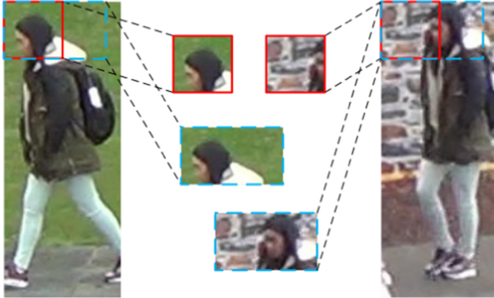
Fig. 1. The problem of a pair images. While the red box of left image can learn the head information, the red box of right image at same location only extracts several valuable information. If the filter changes to rectangle, the two images can gain similar information, as shown as the blue boxes. (For interpretation of the references to colour in this figure legend, the reader is referred to the web version of this article.)
