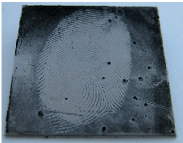
Fig. 2 Sebaceous fingerprint on stainless steel enhanced by PEDOT deposition from EDOT monomer solution containing 1 \text{ mol dm}^{-3} \text{ H}_2\text{SO}_4/0.01 \text{ mol dm}^{-3} \text{ SLS} . Deposition (3500 s) on freshly fingerprinted surface. Viewed ex situ ; Bandey scale grade 3.
