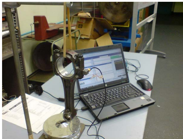
Figure 8. The inertia property measurement of the connecting rod
