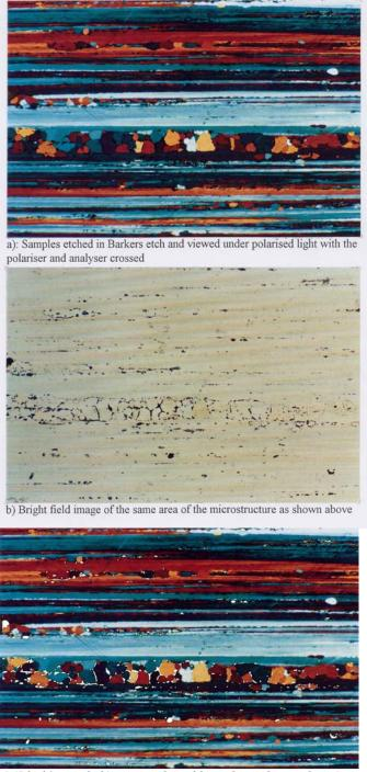
c) 'Black' areas in b) converted to white and superimposed on a).  $100 \mu m$
