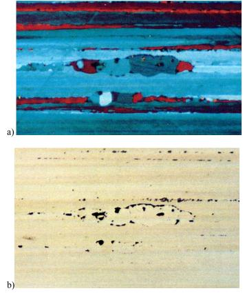
Fig. 4 Higher magnification of Fig. 3 material a) Barkers etch and b) bright field of same area.
