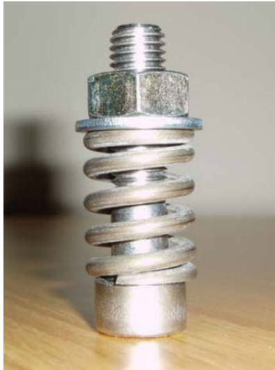
Figure 1: The spring in the bolt assembly. The ends of the springs are flattened and tapered. The spring is subjected to a fixed compressive displacement \delta using a tightened nut and bolt.
