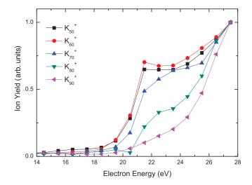
FIG. 1. (Color online) Ion yield curves as a function of electron energy for selected  $K_n^+$  cluster ions (n = 50, 60, 70, 80, and 90). The curves were normalized such that the ion yields are the same at the maximum incident electron energy used (27.5 eV).
