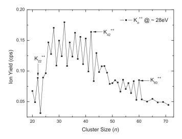
FIG. 5. Ion yield as a function of cluster size n for  $K_n^{2+}$ . Possible magic number ions are identified in the plot.
