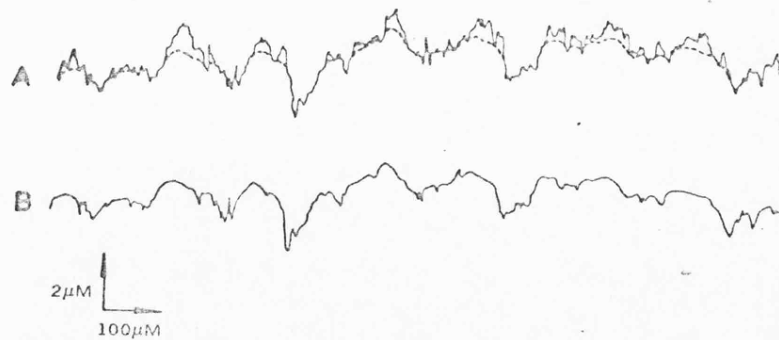
FIG. 11 TALYSURF PROFILES OF CYLINDRICAL SPECIMENS USED IN LUBRICATED FRICTION EXPERIMENTS. (A) Original surface profile (with profile of (b) superposed). (B) Profile of the same line after one traversal of the load. Specimens 0.5% C. steel, 300 D.P.N., 0.635 mm diameter, 32 \times 10^{-6} in. Load 2.5 Kg.
