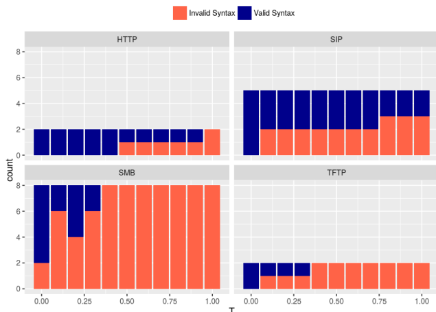
Figure 3. Number of syntactically valid/invalid message patterns - as indicated by Wireshark - in relation to the choice of the generalisation threshold ( T ).
