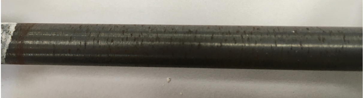
Figure 6.15: Grade 91 typical bolt surface after ~ 1700h and multiple tests.
