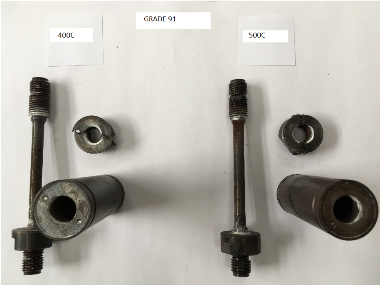
Figure 6.14: Model bolt surfaces at temperature extremes.
