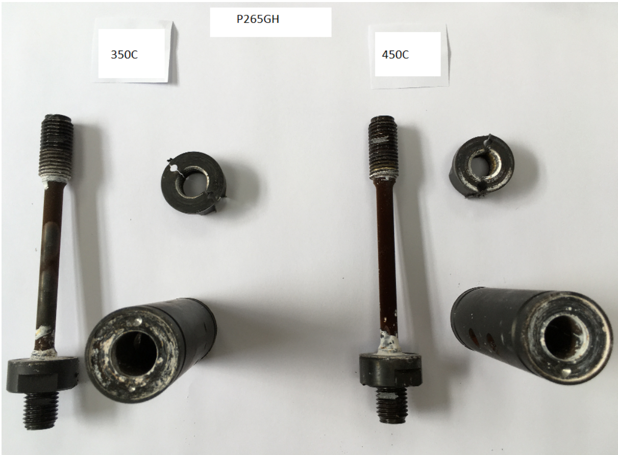
Figure 6.10: MMB surfaces after removal of the nuts by drilling.
