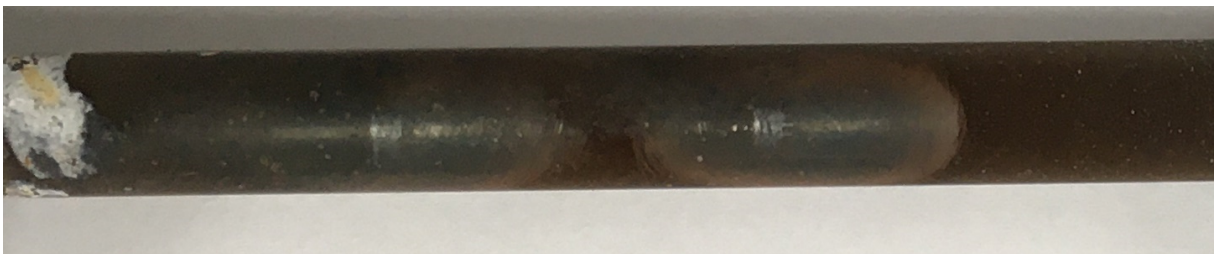
Figure 6.11: P265GH typical bolt surface after 2kh and multiple tests.
