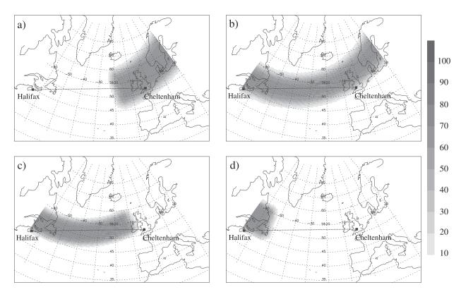
**Figure 1.** Map showing the location of the transmitter at Halifax and receiver at Cheltenham together with the great circle path. The reduction in electron density (expressed as a percentage of ambient) associated with the trough and employed in the ray tracing simulation for the following times is also indicated: (a) 2100 UT, (b) 0000 UT, (c) 0600 UT, and (d) 0900 UT.
