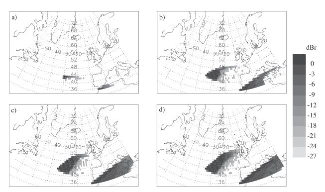
**Figure 4.** The effect of moving the trough in geomagnetic latitude on the relative power of a 10.9 MHz signal at ground level (25 March 1994, 0300 UT). The geomagnetic latitude of the equatorward wall of the trough is (a)  $56.5^{\circ}$ , (b)  $58.5^{\circ}$ , (c)  $60.5^{\circ}$ , and (d)  $62.5^{\circ}$ . The model value [*Halcrow and Nisbet*, 1977] is about 57° (see Figure 1b). 0dBr represents 200 rays landing in an area with sides of 1 degree in both latitude and longitude.
