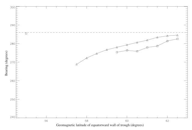
**Figure 5.** Simulated bearing of a 10.9 MHz signal as a function of the position of the equatorward wall of the trough at (a) 0000 UT (triangles) and (b) 0300 UT (squares). The horizontal dashed line indicates the bearing of the GCP.
