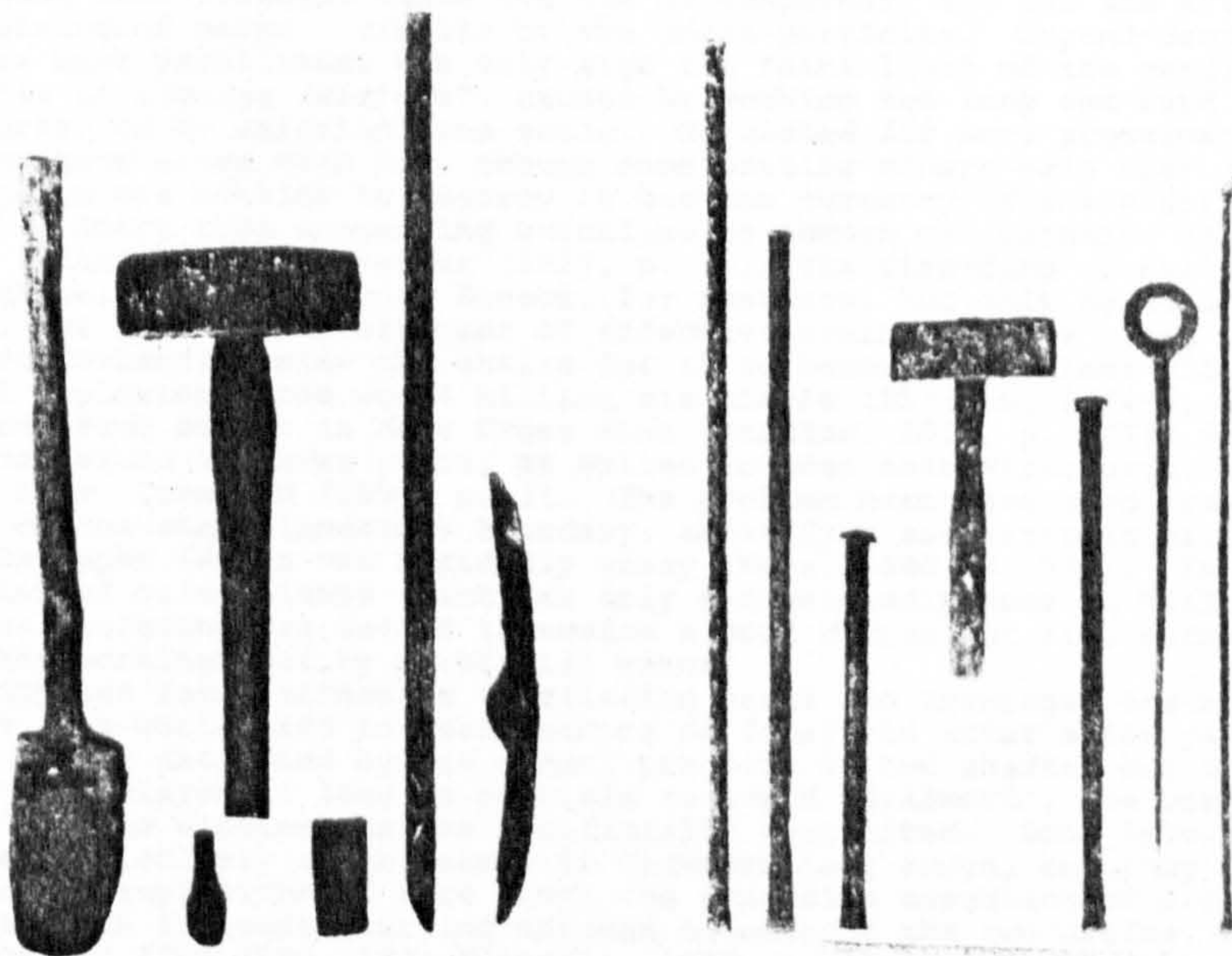
Fig. 3 . (a) Miners tools (from left to right) wooden spade (metal edge missing); scraper; balching hammer; wedge; crowbar and pick.
