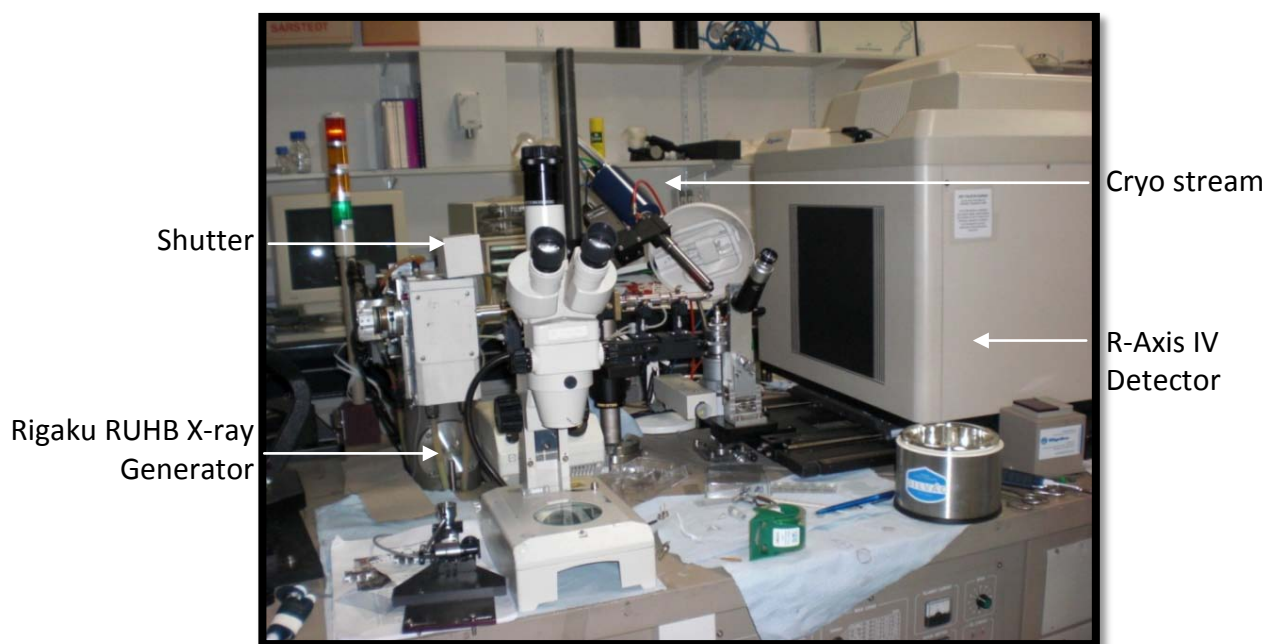
Figure 7.11 A Rigaku RU2HB X-ray generator with a copper anode, Xenocs multilayer optics and an R-Axis IV detector.
