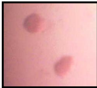
Figure 2.14 TDO crystal attempts, they have some shape and maintain a red colour, however they do not diffract. Protein solution: 50 mM Tris pH 9.0, 5 mM 4-phenyl-imidazole. Well solution: 30-50 mM Tris pH 9.0, 8 % PEG 8K, 4 % ethylene-glycol. Cryo protectant 30 % xylitol 6 .
