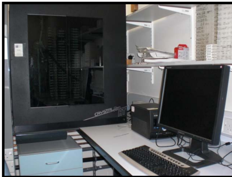
Figure 7.10 CrystalPro® HT (TriTek) a self contained plate storage hotel and imaging robot.
