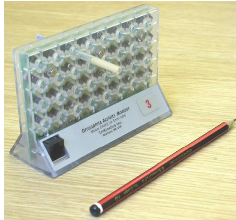
Figure 3-1 Trikinetics DAM5 apparatus loaded with a single activity tube.
