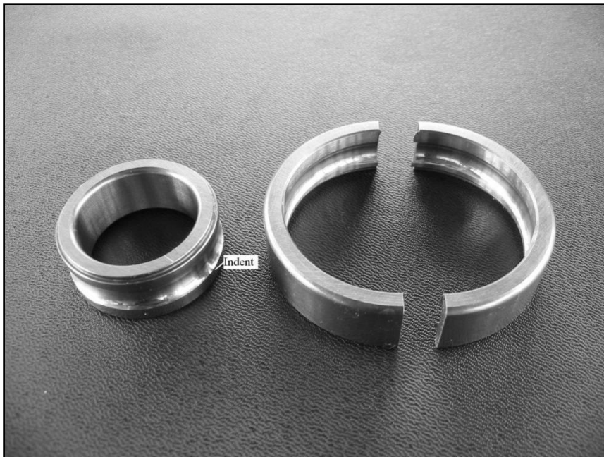
Figure 3-5 Artificially made indent on inner race of bearing.
