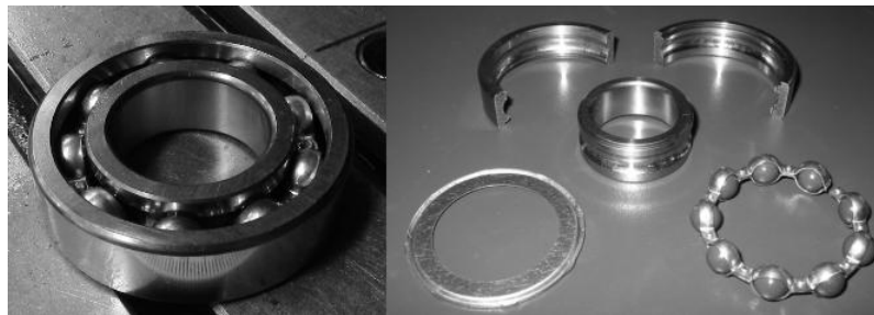
Figure 2-1 A single-row, deep-groove bearing having a shield.
