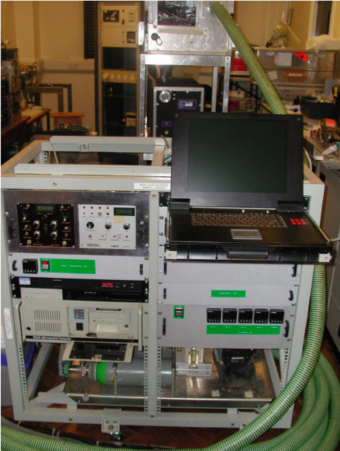
*Figure 2.3 PERCA rack in foreground with inlet box on stand in background, linked by green umbilical*
