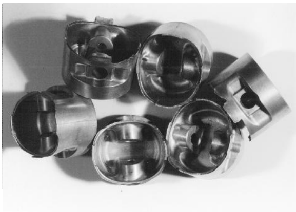
Fig. 8 Pistons thixoformed in the Showa A390 alloy. The biscuit has been machined off and the components washed. Otherwise, these are as-thixoformed.
