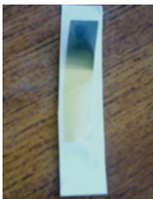
Figure 7.15: Nafion® strip with immobilised Fe 3+ ion having tested 5-ASA
