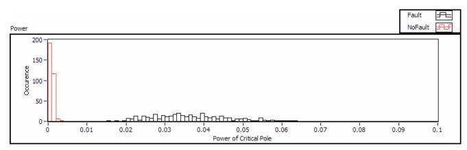
Fig.11. Distribution of Normal and Faulty Poles power parameter. Pole distribution is separated into two distinct regions. No Overlapping of Normal and Faulty Poles. Note these were plotted for frame sizes of 2000 samples. No ROC analysis necessary.
