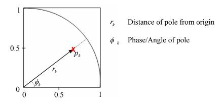
Fig.2. Defining the parameters of an AR pole.
