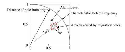
Fig.7. Locus of a particular pole versus evolution of time. Note that pole is migratory and the area pole traverses can be calculated. Alarm level for the characteristic defect frequencies can be determined from standards such as the ISO 10816 and if pole crosses the alarm level, we can conclude that the defect is causing the characteristic frequency and hence the pole displacement is severe.
