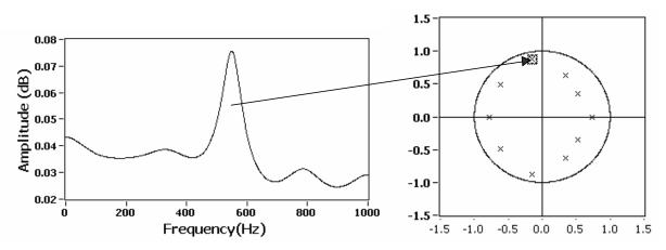
Fig.1. Monitoring the peaks obtained from the AR model. In this case, AR model order was 8 and sampling frequency was 2000 Hz. Notice that it is only the pole nearest to the unit circle that gives rise to a sharp peak in the AR spectrum.
