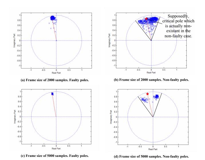
Fig. 10. Distribution of poles from a pump running in normal conditions (right) and for a case with a bearing which has an inner race fault (left). Dotted red line denotes BPFI frequency of 555 Hz. Note concentrated clustering of poles near unit circle for BPFI frequency at approximately 555 Hz for faulty data. Spread of poles is much larger for normal conditions.
