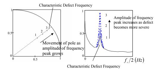
Fig.5. Typical movement of pole as defect becomes more severe (from 1 to 3) and amplitude of vibration of characteristic defect frequency begins to increase.
