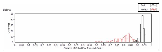
Fig.13. Distribution of Normal and Faulty Poles using distance from the centre of unit circle as the decision parameter. Less overlapping of Normal and Faulty Poles. Note these were plotted for frame sizes of 5000 samples.
