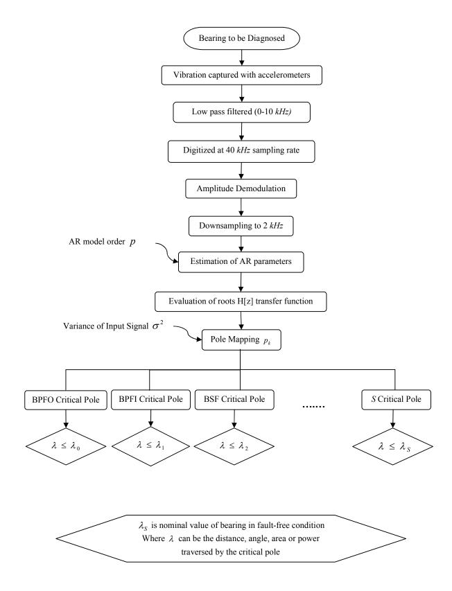
Fig.8. Block diagram of the procedure for bearing fault detection using AR Pole Tracking.
