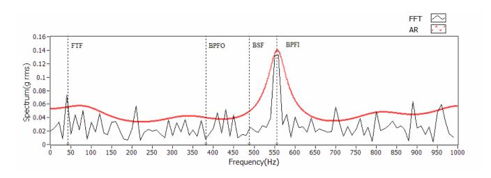
Fig.6. FFT and AR Spectra for ADXL105 vibration signal obtained from a bearing with a seeded inner race fault. Speed of pump was set to 105~Hz. Sampling rate  $f_s$  was 2000 Hz. A sample size of N=4000 samples was used. The BPFI (Ball Pass Frequency of Inner Race) at 556~Hz is clearly evident in both spectra at 555~Hz (lower than theoretical BPFI due to slip- see text). A model order of 10 was used for the AR spectrum.
