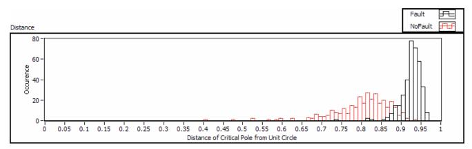
Fig.12. Distribution of Normal and Faulty Poles using distance from the centre of unit circle as the decision parameter. Some overlapping of Normal and Faulty Poles. Note these were plotted for frame sizes of 2000 samples. If bigger sample sizes are used, less overlapping will occur.
