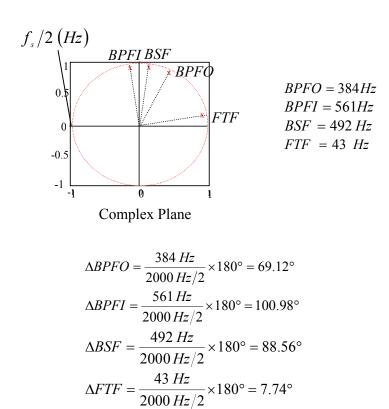
Fig.4. Theoretical location of characteristic defect frequencies in the z plane can be worked out with standard reference formulas if the bearing dimensions are known. Pump was set to  $105\ Hz$  and sampling frequency used was  $2000\ Hz$ .
