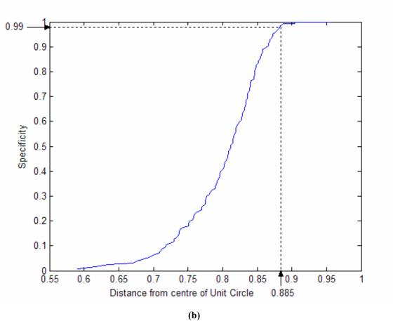
Fig.15. Sensitivity (a) and Specificity (b) curves for a frame size of 4000 samples. Note that distance from centre of unit circle was used as a decision parameter. Even when using the distance as the diagnostic parameter, one can obtain 99 % sensitivity and 99% specificity for frames of 2 seconds duration.
