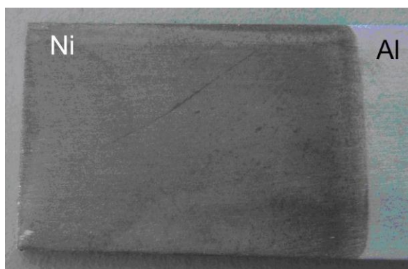
Figure 5.11 Photograph of a nickel layer deposited onto an aluminium substrate following electrolysis of \text{ChCl} : 2 \text{ EG} containing 0.2 \text{ mol dm}^{-3} with 3 mol equivalents of en at an applied potential of -2.5 \text{ V} for 120 min.
