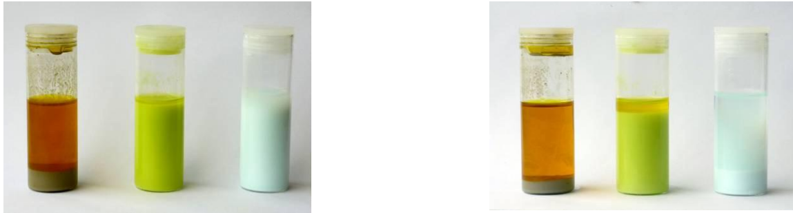
Figure 3.6 Photographs of (from l to r in each photograph) SiC 1-3 µm in EG liquid, Al 2 O 3 0.05 µm in EG liquid and Al 2 O 3 0.05 µm in water. Left after 24 hours and right after 7 days.
