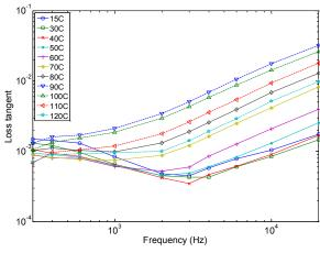
Figure 2 Frequency spectra of cable AAA
