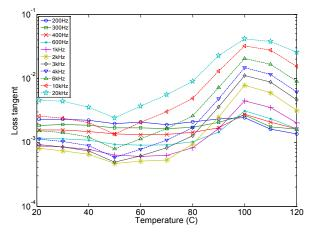
Figure 5 Temperature spectra of cable BAB
