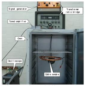
Figure 1 Transformer ratio bridge system setup
