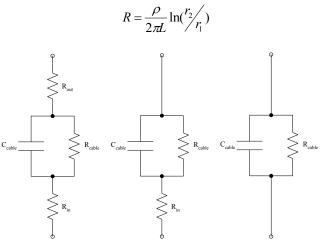
Figure 7 Equivalent circuits of power cables
