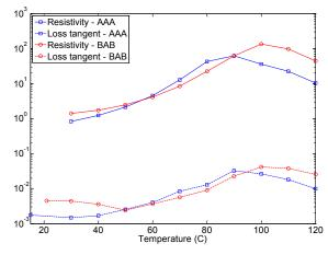
Figure 6 Comparison between resistivity measurement and loss tangent measurement
