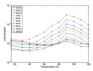
Figure 3 Temperature spectra of cable AAA
