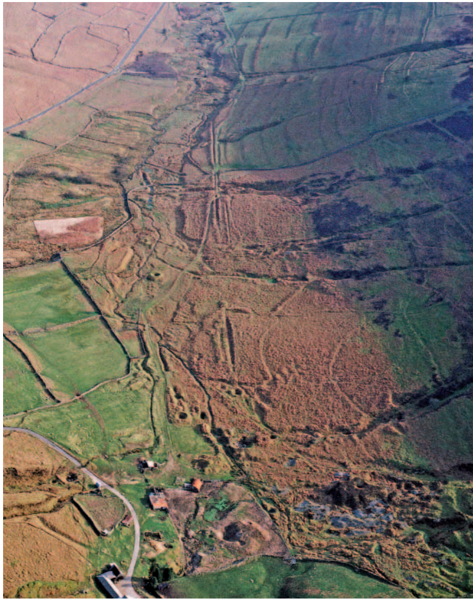
Fig 7.18 Aerial view of East Birch Tor mine showing the flatrod channel running along the valley floor. (NMR 21582/06)
