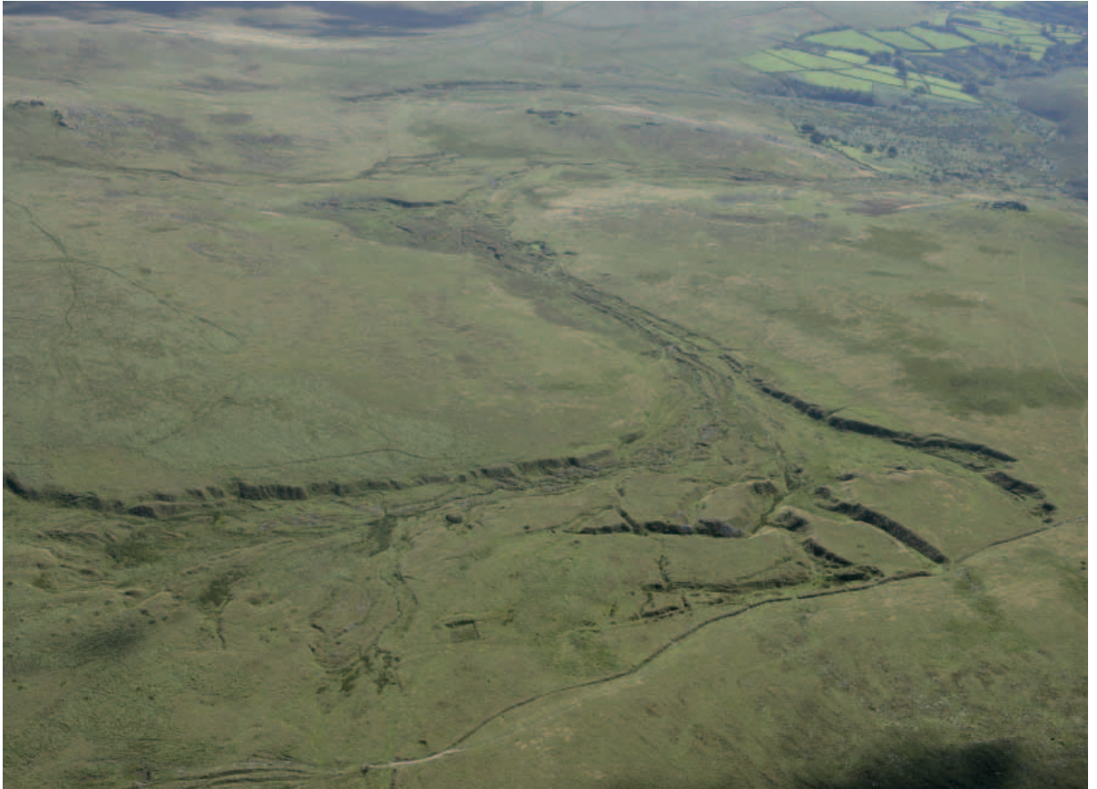
Fig 4.1 Aerial view of Dick's Pits tin streamworks at the head of Doetor Brook showing the extent of disturbance caused by streamworking in a typical upland valley. (NMR 24680/023)
