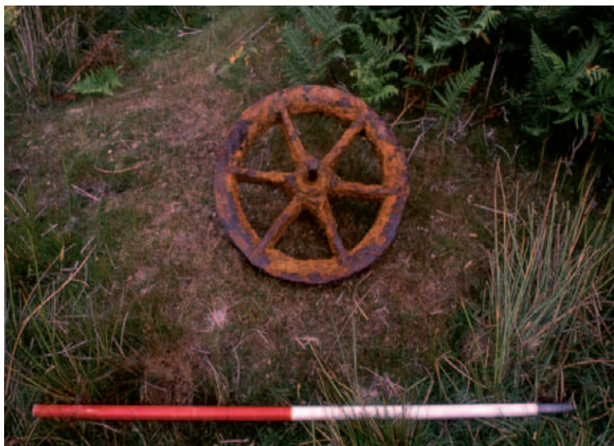
Fig 7.16 A flanged support wheel from the flatrod system at Hexworthy Mine.
