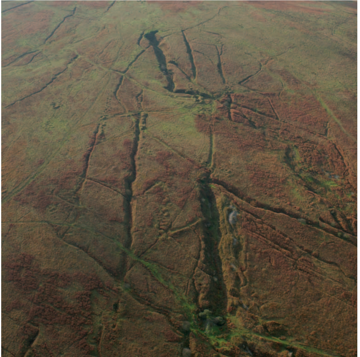
Fig 7.7 Aerial photograph of Ringleshuttes tin mines showing the linear earthworks and streamworks later worked to greater depth using shafts. (NMR 24012/027)
