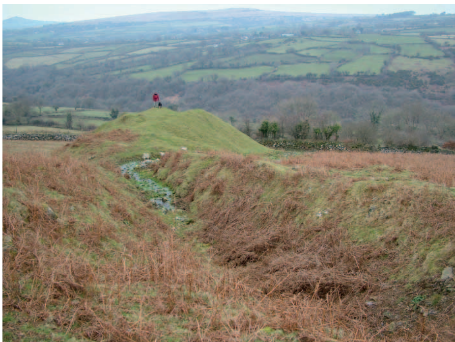
Fig 7.34 A sizeable flat-topped spoil heap made up of mine waste from an unnamed developed prospect on Cudlipp-ton Down. The material emanates from an adit, whose open access gully is visible in the foreground.
