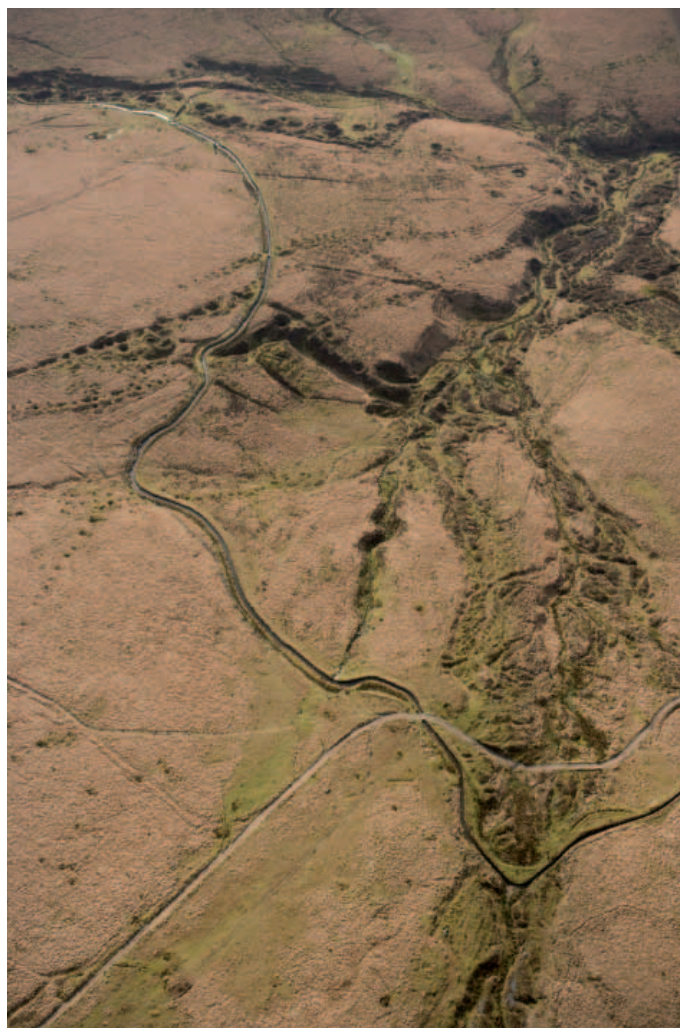
Fig 7.3 Aerial photograph of Newleycombe valley. Shows the areas of tin streamworks following the base of the valley, alignments of prospecting pits, and larger pit workings. Just above centre is a small L-shape openwork which has been penetrated by later shafts. (NMR 24899/031)
