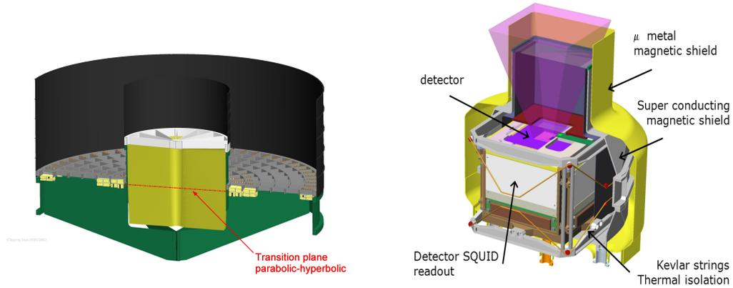
**Fig. 10** Left: Design of the CRIS hybrid mirror. Inner part: classical Ni formed shells mounted on a spider. Outer part: SPO modules (yellow) mounted in four petals (grey). The green part is the structural support. Right: engineering view of the CRIS focal plane assembly
