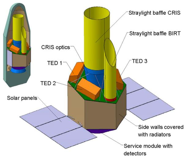
**Fig. 13** Accommodation of the payload and satellite systems in ORIGIN and accommodation in the fairing (top left). The launch mass, including adaptor and margins is 2904 kg and the total power including margin is 2790 W.
