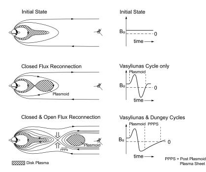
Figure 2. Schematic of three possible states of the magnetotail and the associated  $B_{\theta}$  signatures as measured by a spacecraft situated down the tail.
