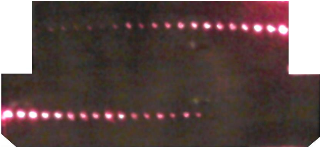
Figure 4.7: Image pattern created on the field mirror, at a distance of 0.8 m from the optical mirror, using a HeNe laser
