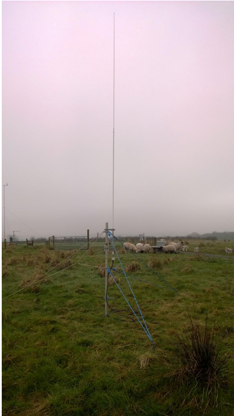
Figure 5.4 Whip antenna at the Lancaster receiving site
