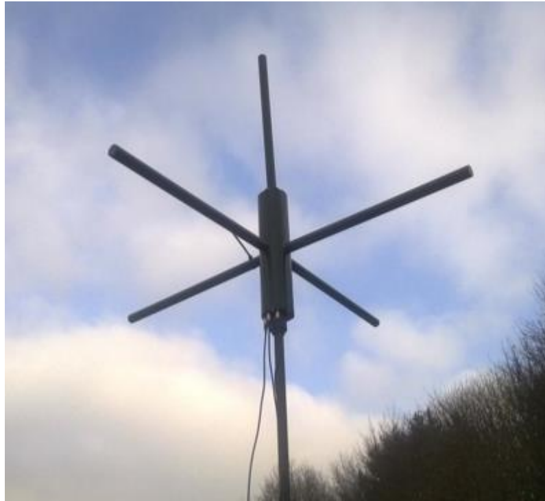
Figure 3.10 Crossed dipole with single monopole receiver antenna array
