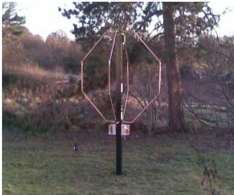
Figure 3.11 Dual perpendicular octagonal loop transmitter antenna array
