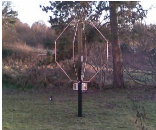
Figure 6.5 Dual perpendicular octagonal loop transmitter antenna array
