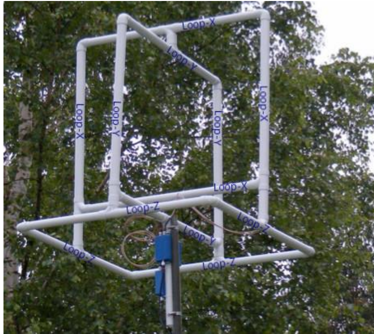
Figure 3.8 'X-Y-Z' Loop receiver antenna array
