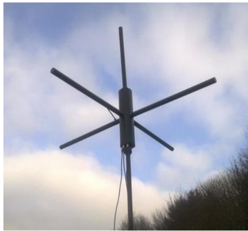
Figure 6.6 Crossed dipole with single monopole receiver antenna array
