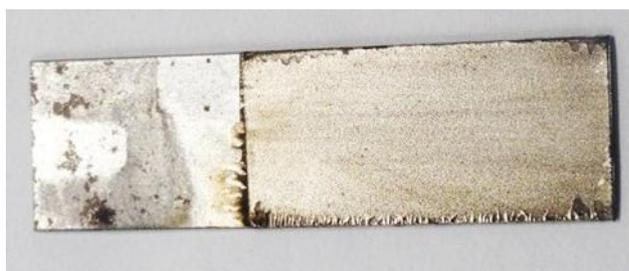
**Figure 10:** Photograph of a nickel layer deposited onto a mild steel substrate following electrolysis of  $\text{ChCl: 2 EG}$  containing  $1.14 \text{ mol dm}^{-3}$  at  $80 \text{ }^\circ\text{C}$  and current density of  $1.5 \text{ A dm}^{-3}$  for 1 h. The substrate was etched in-situ by applying  $1 \text{ A dm}^{-2}$  for 30 sec.
