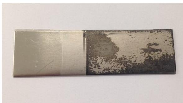
**Figure 2:** Scanning electron micrograph (*left*) with a corresponding photo image (*right*) of the nickel coating resulting from electrodeposition at a driven current density of  $1.5 \text{ A dm}^{-3}$  for 1 hour in a  $1.14 \text{ mol dm}^{-3}$  solution of  $\text{NiCl}_2 \cdot 6\text{H}_2\text{O}$  in Ethaline at  $25 \text{ }^\circ\text{C}$ .
