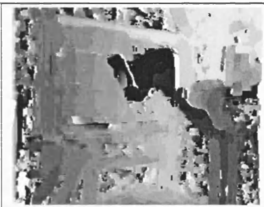
Figure (4.2f) – Pseudo-normalised correlation using a 9x9-pixel correlation window.
