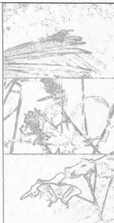
Figure (6.8c) – The result of applying a 9x9 binary Laplacian filter to figure (6.8a). All edges above threshold were set to a pixel intensity of 153 (out of 0-255).
