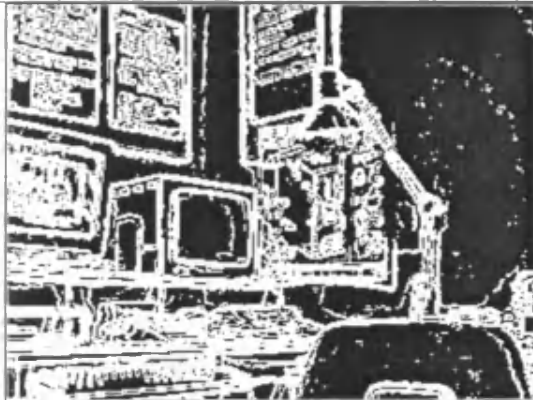
Figure (3.12e) – Sobel edge operator (equation [3.13] & [3.14]) with properties as for figure (3.12c).
