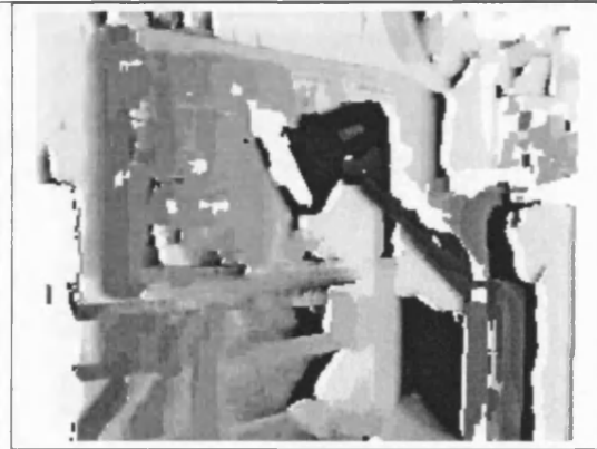
Figure (4.2d) – Sum of squared differences with a 9x9-pixel correlation window.
