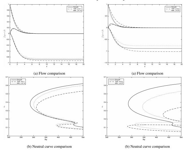
**Figure 1.** Model comparison at a = 0.1 and  $\eta = 0.14$ .
