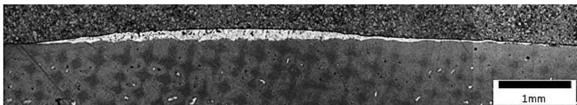
Figure 2.5 OM image of melt blister cross-section from a heat-treated SX turbine blade
