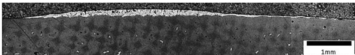
Figure 4.2 OM image of melt blister cross-section from a heat-treated SX turbine blade
