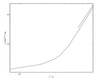
FIGURE 8. A comparison between the scaled effective asymptotic Taylor number  $\bar{T}$  (above) and the Reynolds number Re predicted by the Orr-Sommerfeld analysis (below), against vortex wavenumbers  $\epsilon^{-1}$  and  $\sigma$  respectively, for  $\psi = 30^{\circ}$ ,  $\phi = 2.7^{\circ}$ .
