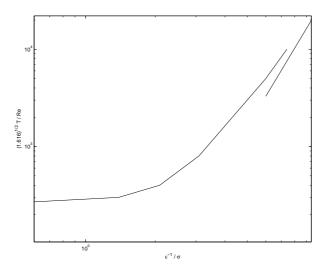
FIGURE 9. A comparison between the scaled effective asymptotic Taylor number  $\bar{T}$  (below) and the Reynolds number Re predicted by the Orr-Sommerfeld analysis (above), against vortex wavenumbers  $\epsilon^{-1}$  and  $\sigma$  respectively, for  $\psi = 45^{\circ}$ ,  $\phi = 8.5^{\circ}$ .
