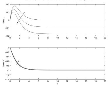
FIGURE 5. Effective velocity profiles  $\tilde{U}$  and  $\tilde{V}$  for waveangles  $\phi = 0^{\circ}$ ,  $5^{\circ}$  and  $10^{\circ}$  (in direction of arrow).
