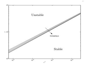
FIGURE 6. Asymptotic scaled Taylor number  $\bar{T}$  as a function of non-dimensional vortex wavenumber  $\epsilon^{-1}$  for  $\phi=0^{\circ}-10^{\circ}$  in increments of 2.5°. The unstable region is above the neutral curves.
