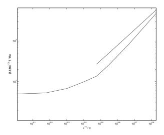
FIGURE 7. A comparison between the scaled effective asymptotic Taylor number  $\bar{T}$  (above) and the Reynolds number Re predicted by the Orr-Sommerfeld analysis (below), against vortex wavenumbers  $\epsilon^{-1}$  and  $\sigma$  respectively, for  $\psi = 15^{\circ}$ ,  $\phi = 0^{\circ}$ .
