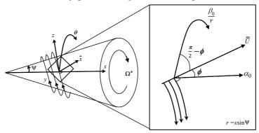
FIGURE 4. Diagram of spiral vortex instability of a rotating cone (left) and the detailed physical interpretation (right) showing streamwise, azimuthal and effective velocity directions. Note that  $\alpha_0$  and  $\beta_0/r$  refer to wavenumbers in the streamwise and azimuthal directions of the previous formulation Garrett *et al.* (2009).
