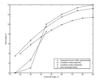
FIGURE 10. A comparison between experimental observations and theoretical predictions of the vortex orientation angle at the onset of instability, updated from Garrett *et al.* (2009). The diagram illustrates the competing nature of the type I (crossflow) instability versus the new (centrifugal) instability modes, which dominate for slender half-angles and compare well with the experimental measurements in this regime.
