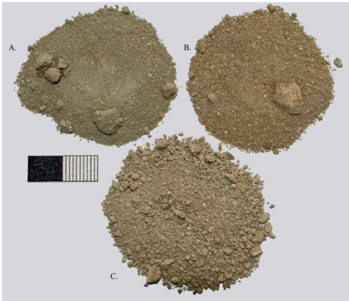
Figure 5.47 Fired tan clays from Agii Pantos Gorge (sample 18) and Periferiaki Aerodromiou Sitias (Greek National Road-E75) (samples 19, 20) broken apart after nine months due to spalling.
