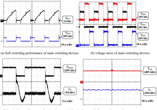
(c) Soft switching performance of active clamp switching devices (d) Output voltage and input current
