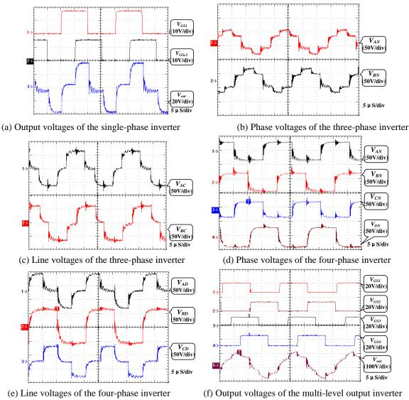
Fig. 15 Experimental results for the proposed inverters.
