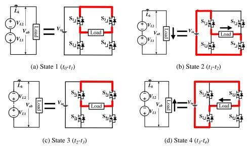
Fig. 4 Operating states of the proposed single-phase inverter
