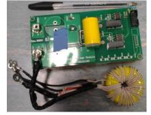
Fig. 14 Photograph of one converter arm.
