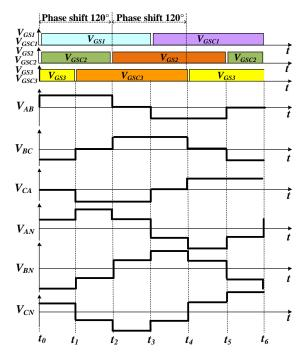
Fig. 6 Output waveforms of the proposed three-phase inverter.
