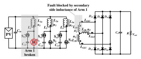
Fig. 11 Fault tolerance under a fault in the primary-side switching device.
