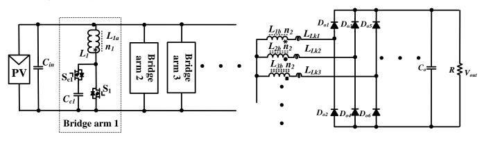
Fig. 12 Expandable characteristic of proposed converter.
