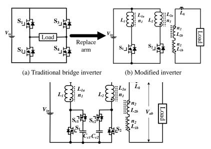
(c) Proposed inverter with an active clamp circuit Fig. 2 Traditional and proposed single-phase inverters.
