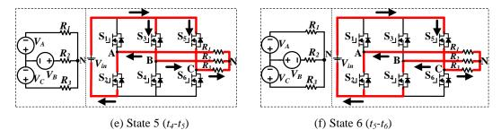
Fig. 7 Six operating states of the proposed three-phase inverter.
