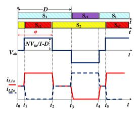
Fig. 3 Output waveforms of the proposed single-phase inverter.
