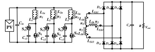
Fig. 10 Front-end topology for PV applications
