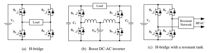
Fig. 1 Common H-bridge inverter topologies.
