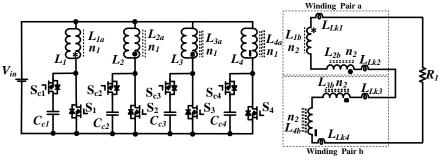
(b) Three-level inverter Fig. 8 New topologies derived from the proposed inverter.
