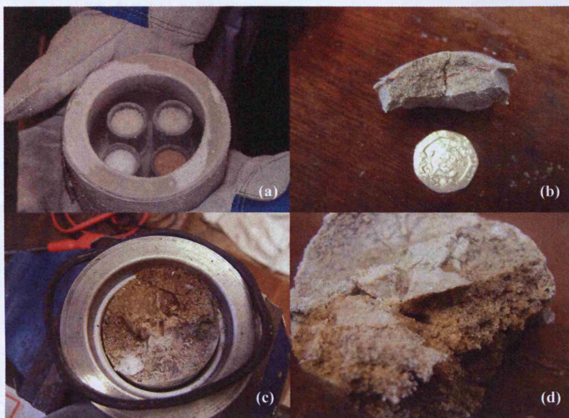
Figure 4.2(a) Image of pressure vessel containing 4 plastic tubes initially completely filled with seawater ice ball/sediment mixes at the start of the experiment. (b) Sediment/CO 2 hydrate sample with a domed base (top of sample in image) due to the lack of a firm base during the experiment (sediment and water placed on a fine mesh). Surface is uneven, and hydrate appears to fill pores and cement grains. (c) Pressure vessel containing sample with a very disturbed surface texture after depressurisation. (d) Sample from (c) with a surface water ice layer and some hoar frost. Some of the sample was completely un-cemented; hence some surface sediment has been lost. Natural sediment also appears fairly porous, and clay sediment appears very disturbed with a very porous texture.
