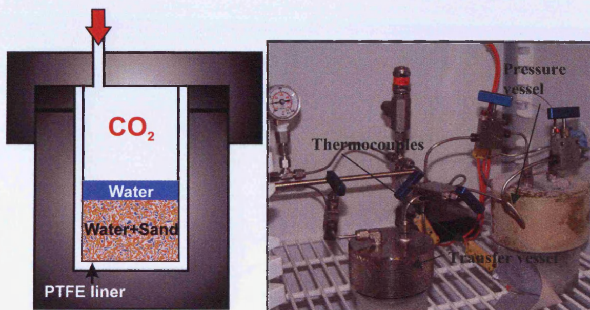
Figure 4.1(a). Schematic diagram of a simple batch experiment; with water and sand in a PTFE liner inside a stainless steel pressure vessel, which when sealed was pressurised with \text{CO}_2 . (b) Image of batch experiments inside the cooled incubator. Various pressure release valves and tubes are added to the experimental pressure vessels for connection and safety.
