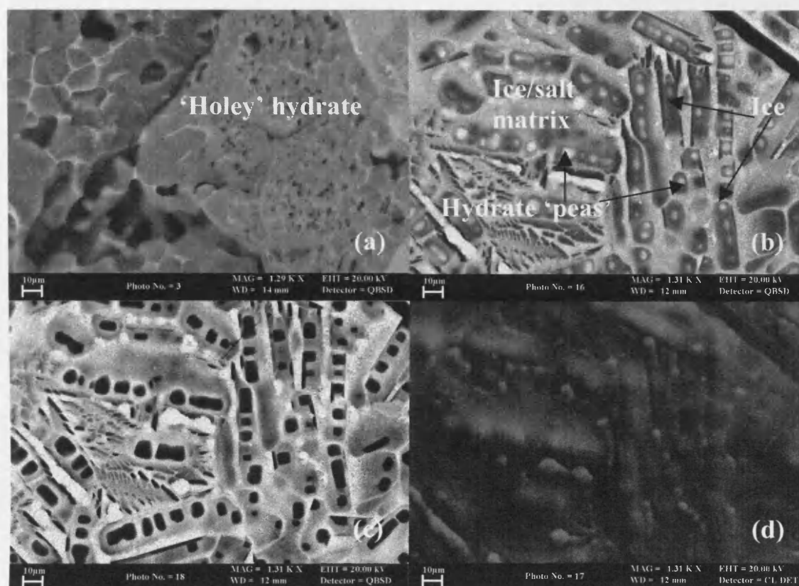
Figure 5.7(a) BSEM image of 'holey' hydrate within a CO 2 hydrate 'curl' found on the surface of sample 2. Sample stage was maintained at approximately -171 °C. (b) BSEM image of 'Pea-pod' hydrate with each pod (c. 40 µm) constructed by spherical and cubic polyhedral CO 2 hydrate 'peas' (<5 µm) surrounded by a layer of ice, another layer of hydrate and then an external ice/salt matrix. (c) BSEM image of (b) after etching at -140 °C. The CO 2 hydrate 'peas' have been ablated during warming, indicating a more unstable hydrate phase. (d) CL image of (b) showing the different phases which seem to be present. Saline regions appear white and water ice appears as darkest grey regions (between other phases).
