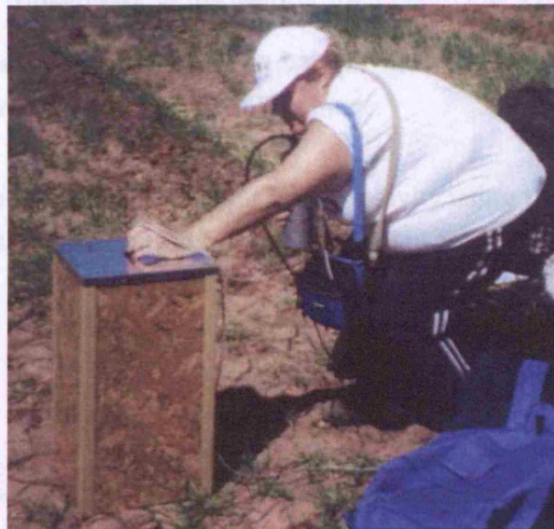
FIGURE 5.6. Collection of radiometric data in field B123 from which surface emissivities are derived using the emissivity box.
