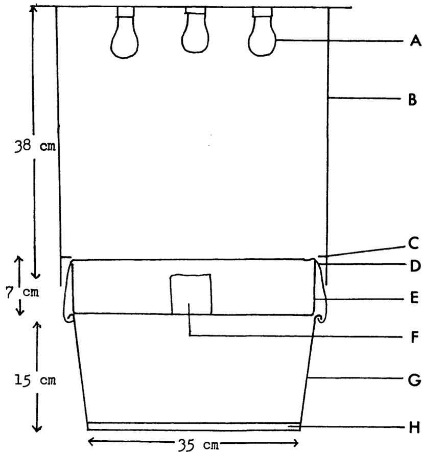
Fig. 2.11 The modified Kempson, Lloyd and Ghelardi extractor, in section.
