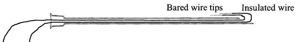
Figure 3.7: Fine wire electrode and insertion needle for relatively painless, detailed and deep muscle electromyography.
