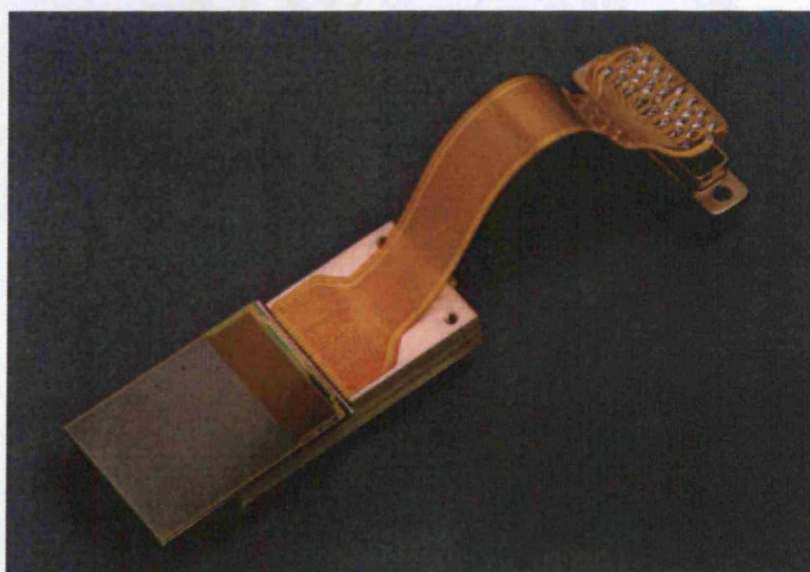
Figure 7-7. CCD22 mounted on three-sides buttable package. All connections are made via the flexible, thermally isolating Kapton circuit (Photo F. Balam).
