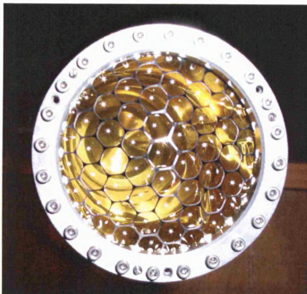
Figure 7-15. Honeycomb support structure on the end of the target cell.
