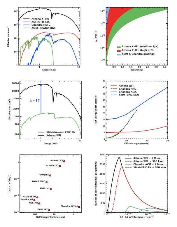
**Figure 1**. From top left to bottom right, *Athena* performance vs earlier missions: (a) effective area for high-resolution spectroscopy; (b)  $L_X$ -z parameter space available for high-resolution spectroscopy; (c) effective area for imaging and medium-resolution spectroscopy; (d) spatial resolution at various off-axis angles; (e) survey grasps and (f) survey speed in sources per pointing
