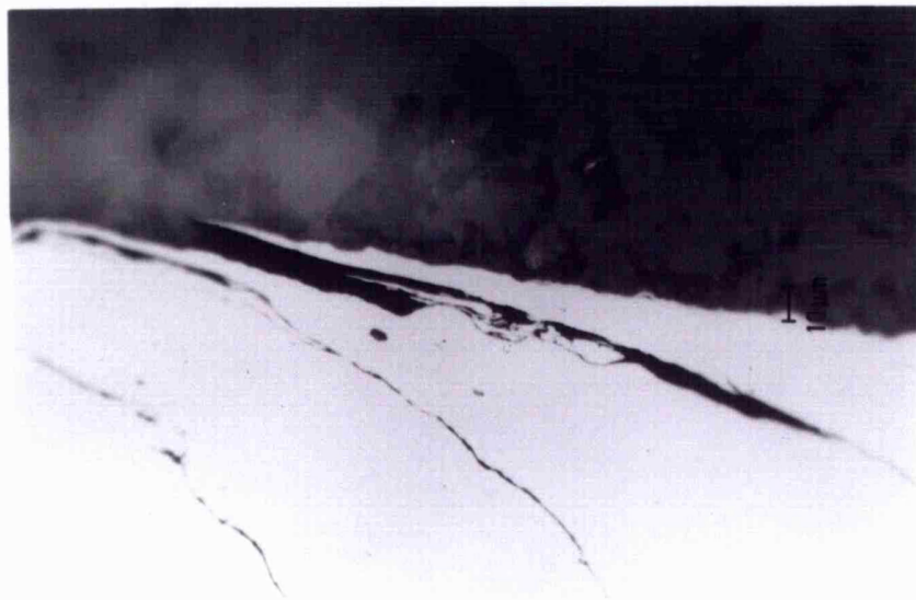
(b): RCF CRACK MOUTH CAUSED BY A DRY-WET CYCLING REGIME OF 500 DRY FOLLOWED BY 26119 WET ROLLING-SLIDING CYCLES (TEST 146 OF TABLE (8.2))
