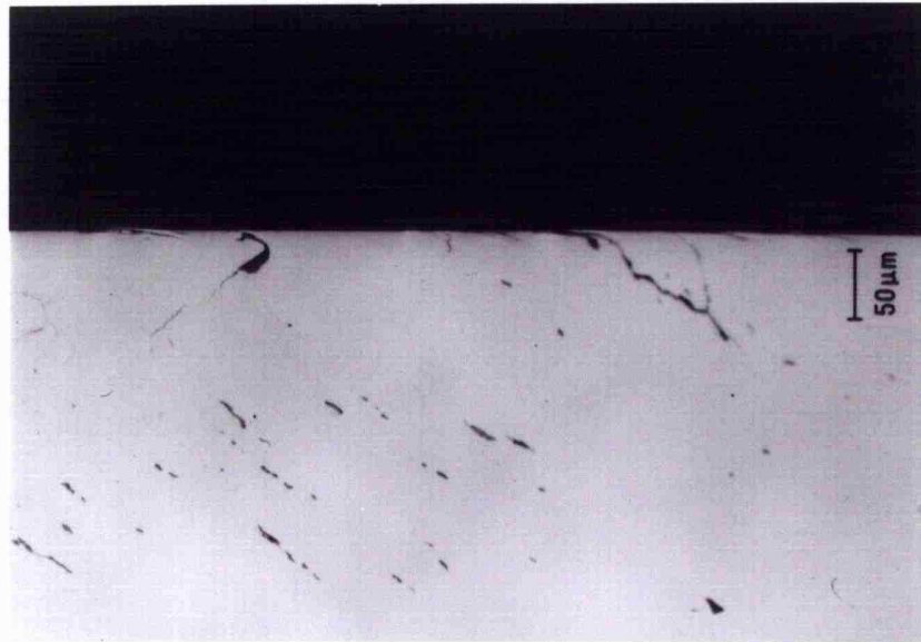
FIGURE (7.7): DOUBLE RCF CRACKING UNDER A REVERSAL FACTOR OF 0.267, TEST NUMBER 115
