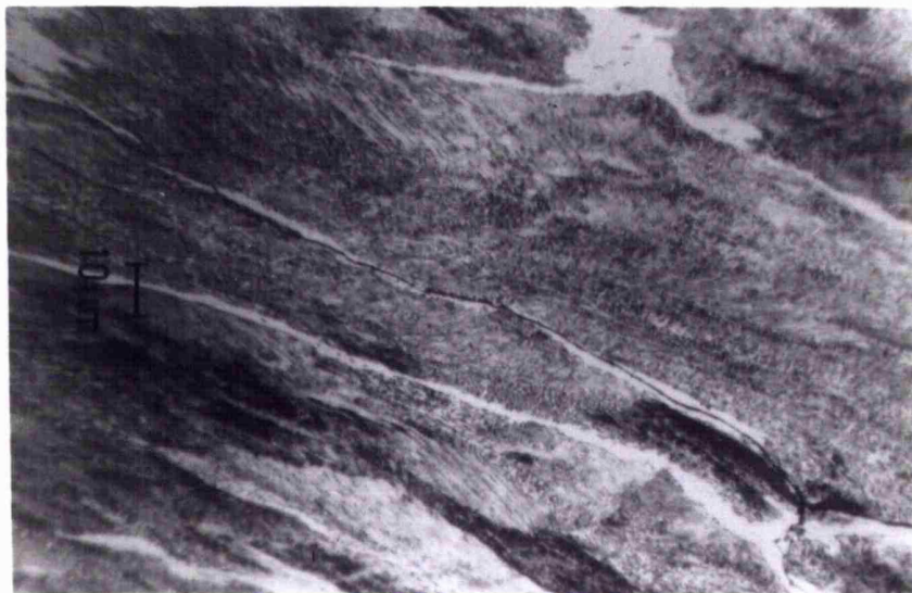
FIGURE (6.10): RCF PROPAGATION THROUGH THE SOFT FERRITE PHASE, TEST NUMBER 114
