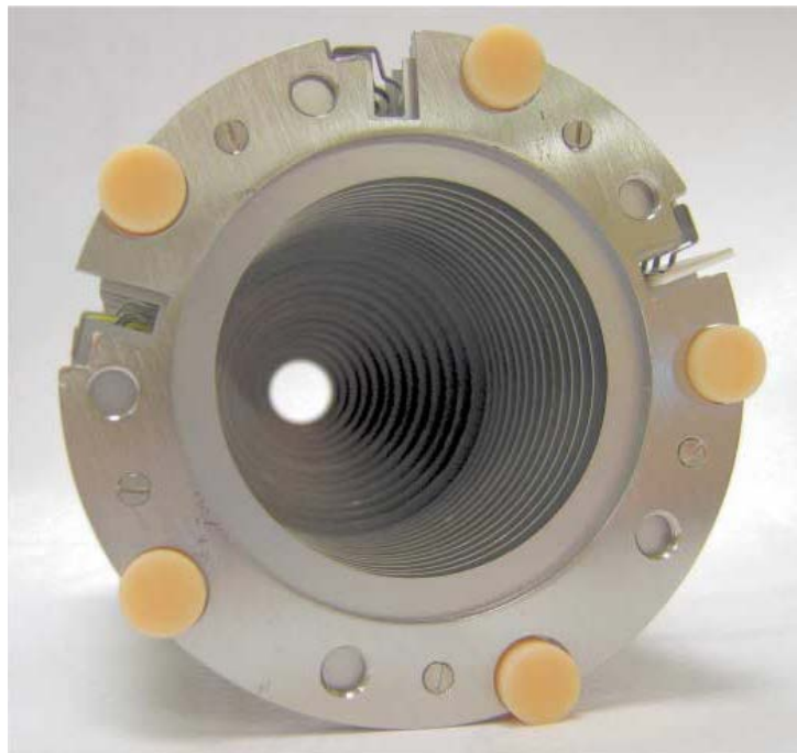
Figure 3-1. Image of ion funnel electrodes with a large diameter tapering down to a smaller internal diameter. The 5 ceramic support rods can also be seen.
