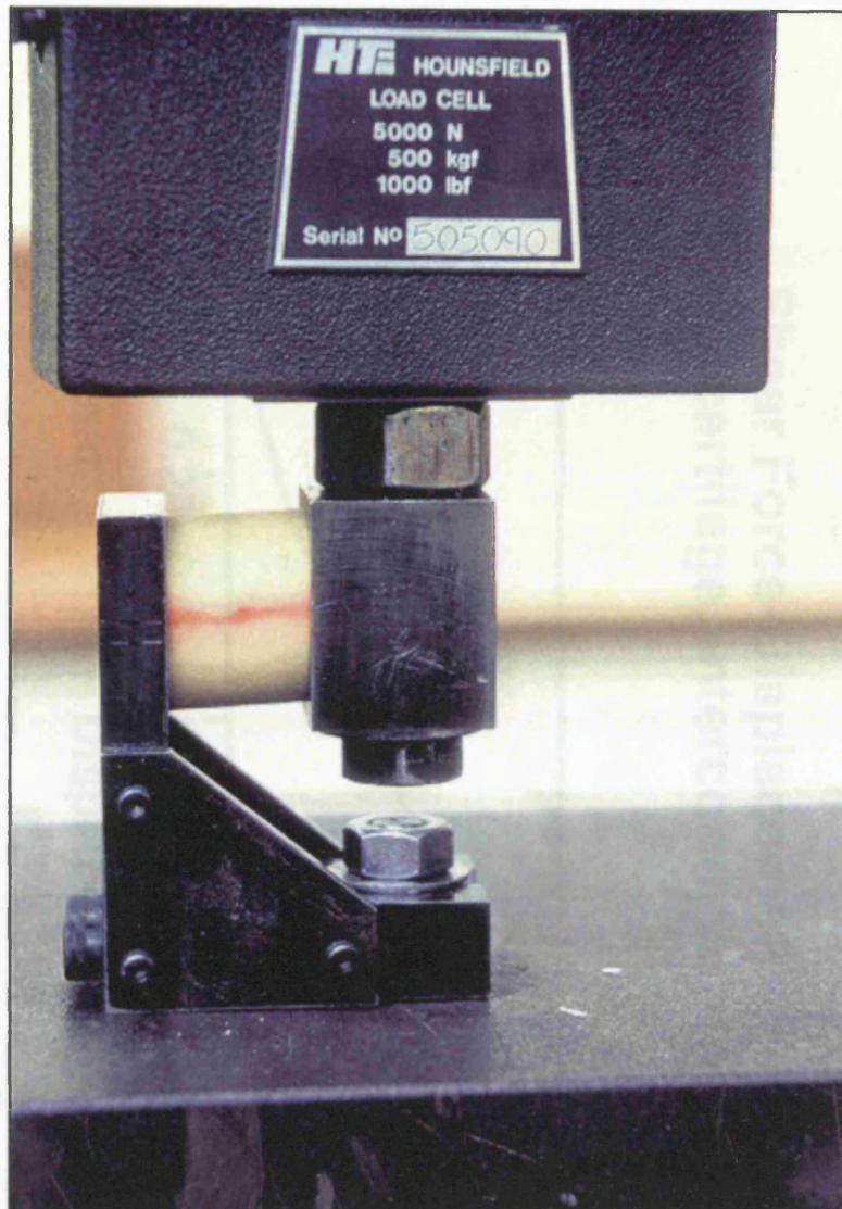
Figure 19 - Photograph of shear apparatus attached to material testing machine.
