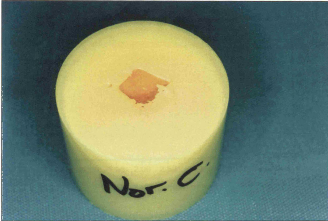
Figure 16 - Photograph showing a specimen embedded in resin.
