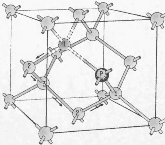
**Figure 6.24** The silicon lattice containing an E-centre defect. The vacancy can reorient itself from its normal position nearest the phosphorous atom to a new nearest site by moving through the lattice as shown
