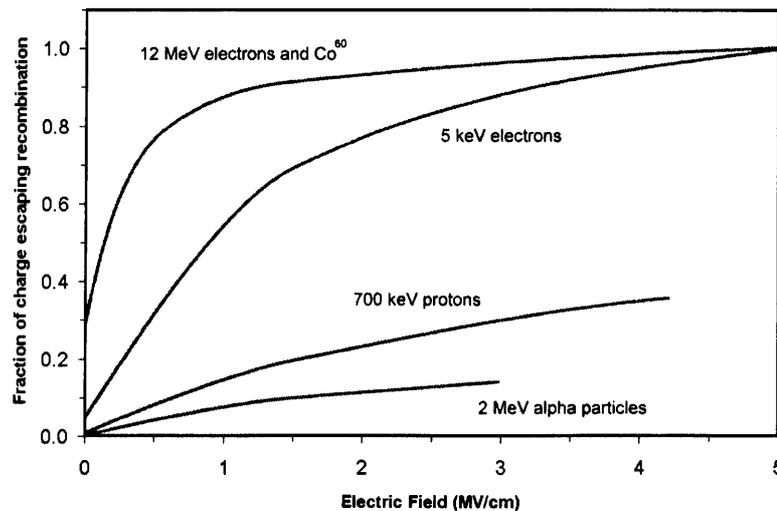
**Figure 3.12** The amount of radiation induced charge escaping recombination at different irradiation bias levels (Robbins 1992)
