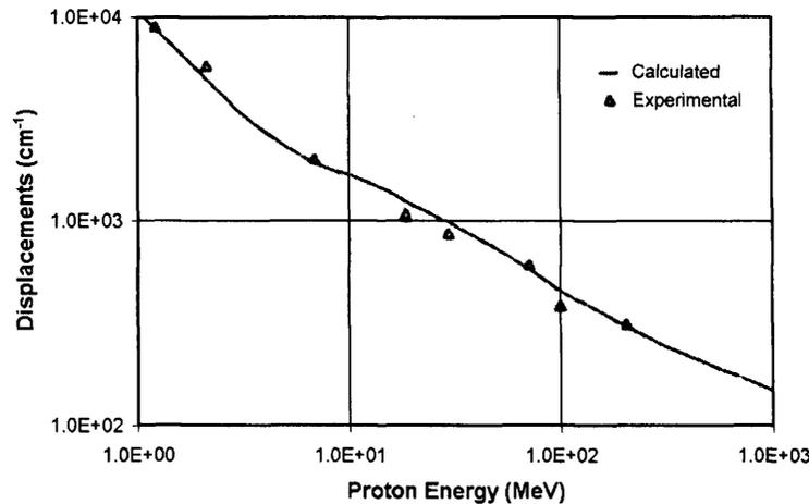
**Figure 3.13** The number of atoms displaced by different energy protons in silicon (Van Lint 1987)
