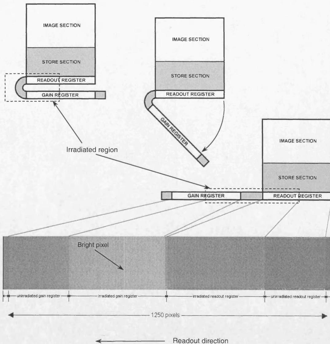
**Figure 4.8** An image taken using a sequencer program that only reads out pixels in the readout and gain registers of the device. The irradiated and unirradiated sections of the readout register can be seen, along with under and overscan pixels. The figure includes diagrams of the L3Vision device to correlate the sections of the recorded image with the physical sections of the device
