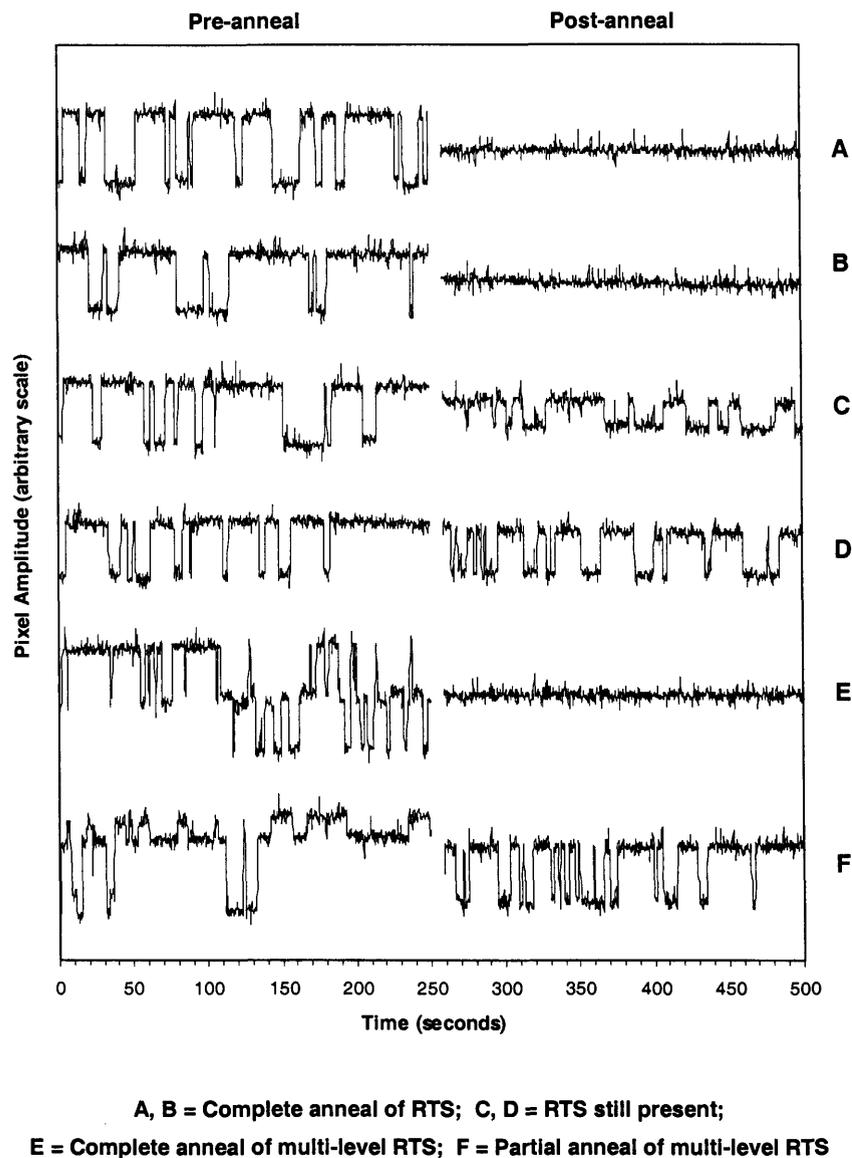
**Figure 6.21** The amplitude variation with time of RTS pixels monitored before and after annealing. The amplitude scale is arbitrary to allow the presentation of the data, however the relative amplitude scale of each data set is the same
