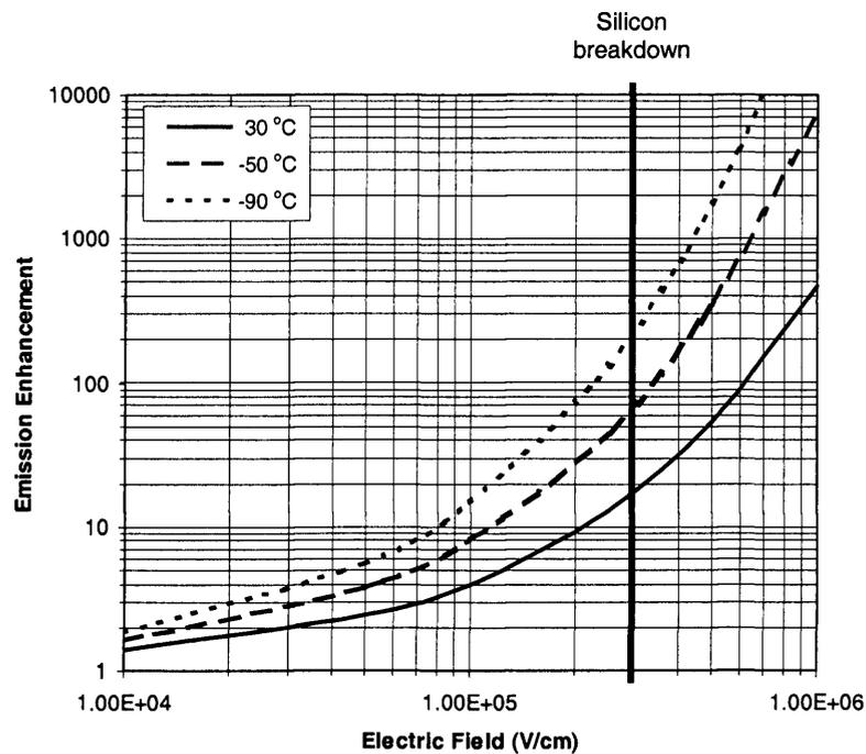
**Figure 3.19** Modelled Poole-Frenkel emission enhancement for silicon
