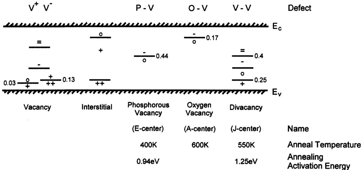
**Figure 2.2** A diagram of the main defect complexes that form as a result of displacement damage in CCDs. Details of the energy levels induced in the silicon band-gap and the approximate annealing temperatures and activation energies are given. The energy levels are in eV measured from the nearest band edge
