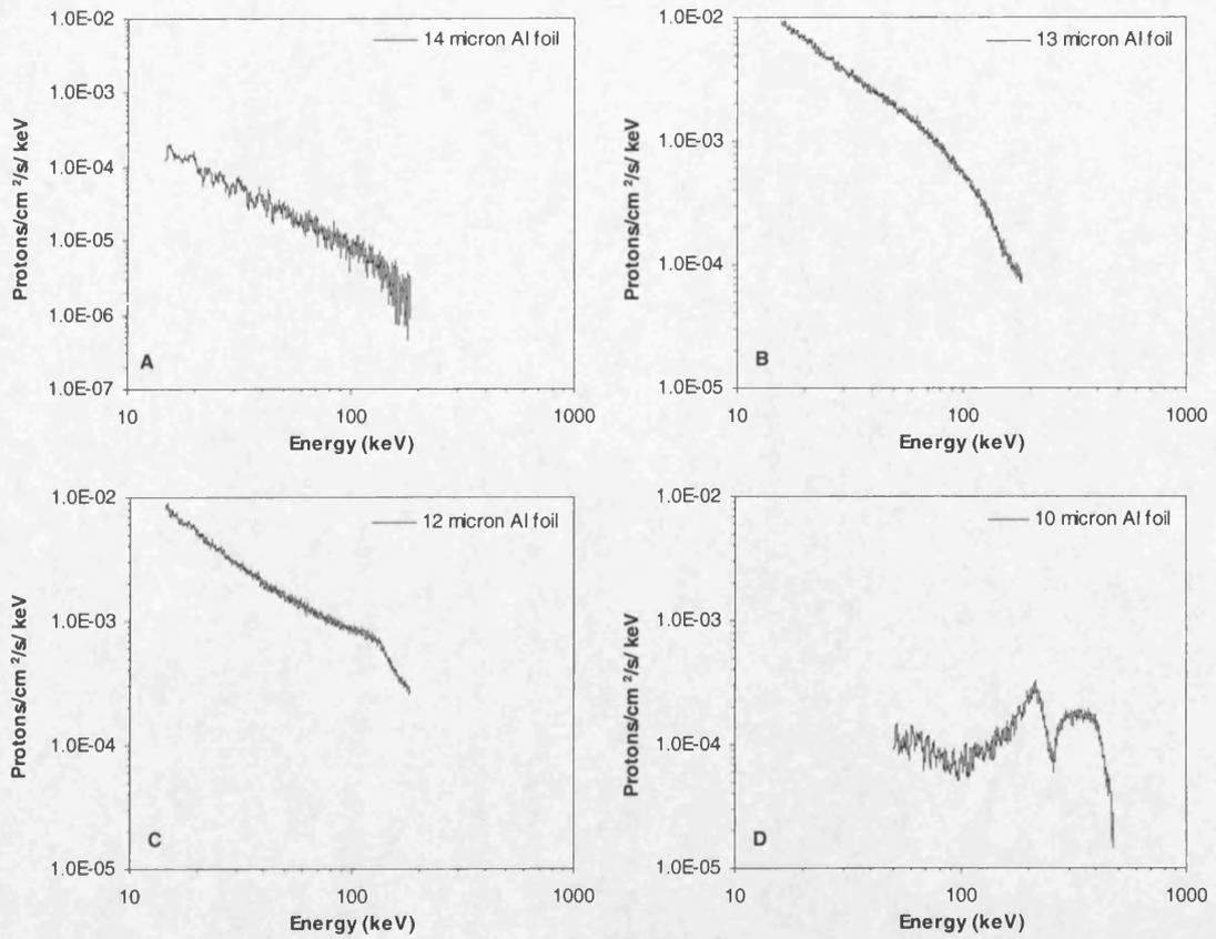
**Figure 5.6** Proton spectra measured with EPIC MOS CCDs after irradiation through four different aluminium foil thicknesses
