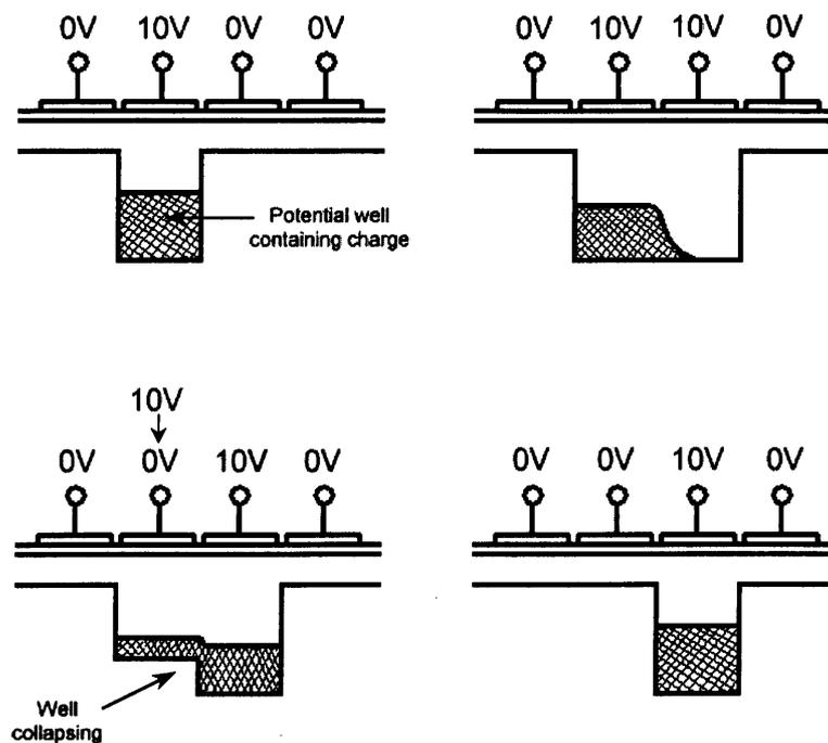
Figure 2.10 The charge transfer process
