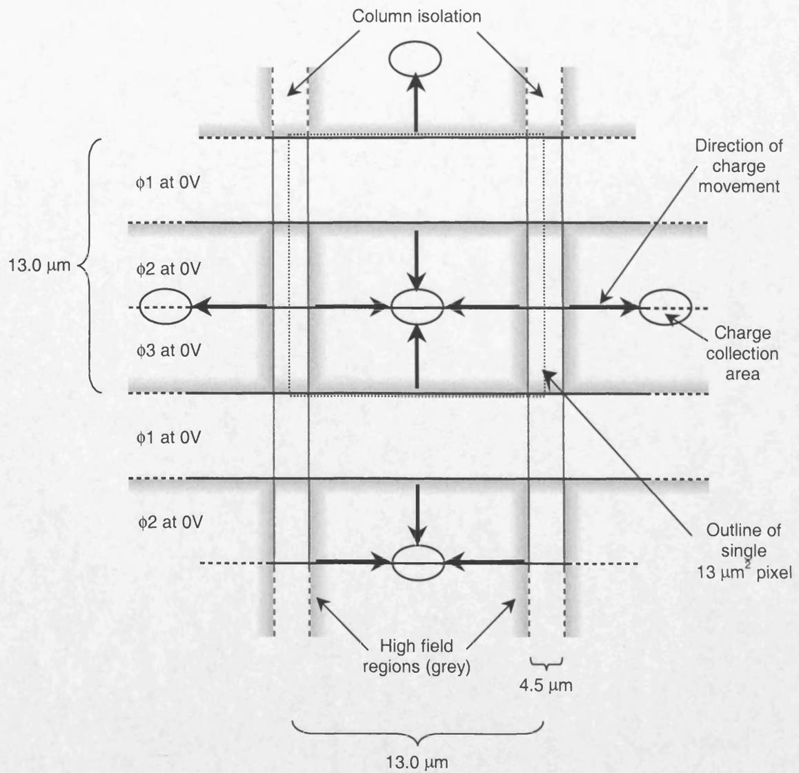
**Figure 6.13** The structure of a CCD47-20 pixel indicating the inter-electrode and channel stop high field regions and the movement of charge into the charge storage region of each pixel
