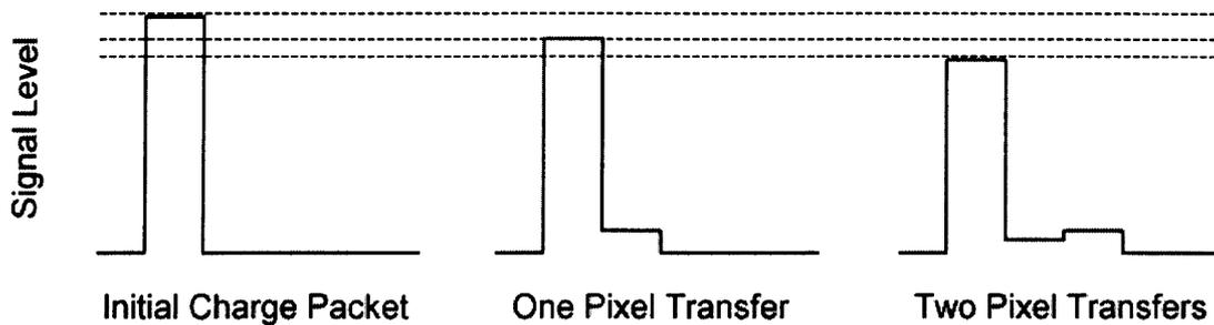
**Figure 2.11** The effect of CTE on a charge packet. Signal charge is lost from the initial charge packet during transfer and is emitted into subsequent pixels
