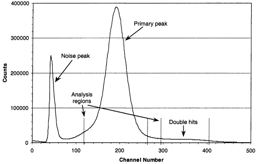
**Figure 4.6** A PIN-3CD photodiode pulse height spectrum
