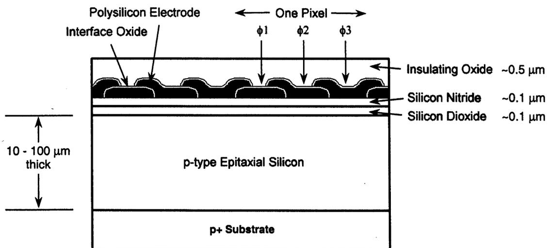
**Figure 2.3** A cross-section through a surface channel CCD showing the 'overlapping' polysilicon electrode structure
