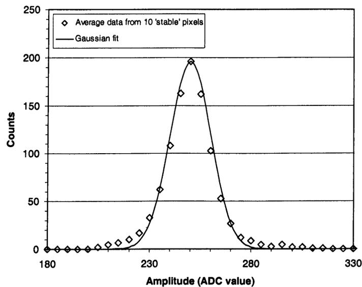
**Figure 6.8** The average amplitude spectrum of 10 'stable' CCD pixels fitted with a Gaussian function. The fit shown has a  $\sigma$  of 10 and was used as the matched Gaussian in the RTS analysis software
