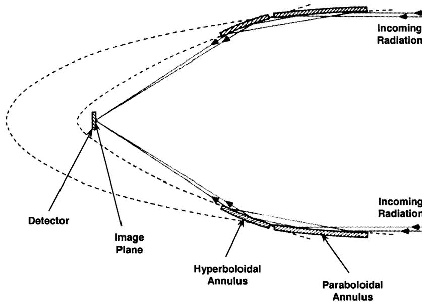
**Figure 5.1** The Wolter Type 1 optic arrangement used for the mirror modules of the Chandra and XMM-Newton spacecraft
