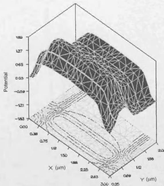
**Figure 2.8** The potential profile under two CCD electrodes in a surface channel device, one biased, one unbiased, modelled using the EVEREST Device Modelling Software for Charge Generation Events (Fowler et al. 1998)
