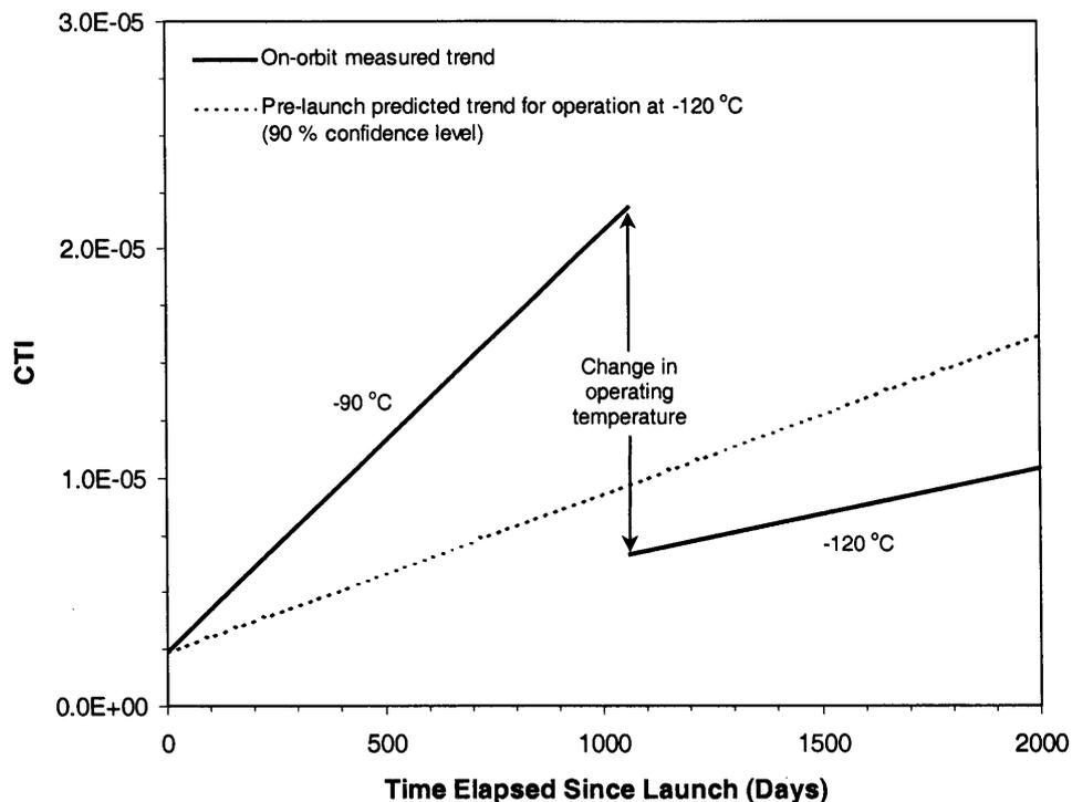
**Figure 5.12** The pre-launch predicted and on-orbit measured Mn-K $\alpha$  parallel CTI change over time for the CCDs of MOS2
