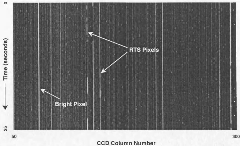
**Figure 6.7** An image taken using a sequencer program that only reads out pixels in a selected row of the CCD. Each row in the image is recorded at 0.25 second intervals revealing the change in amplitude over time of RTS pixels
