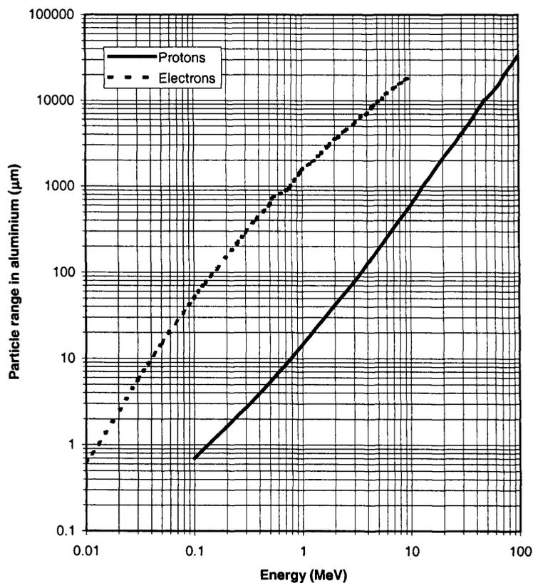
**Figure 3.9** The range of protons and electrons in aluminium (Ziegler et al. 1985)
