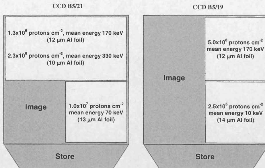
**Figure 5.5** Total doses given to each section of the irradiated CCDs
