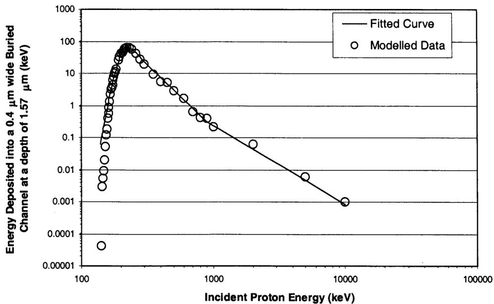
**Figure 5.7** The amount of energy deposited into a 0.4  $\mu\text{m}$  wide buried channel at a depth of 1.57  $\mu\text{m}$  from the surface of a representative CCD22 structure as a function of interacting proton energy
