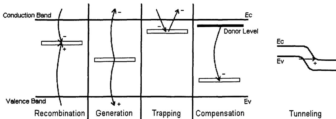
**Figure 3.14** The possible effects of radiation induced levels in the silicon band-gap
