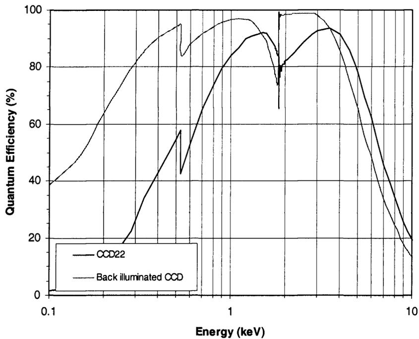
**Figure 2.14** Quantum efficiency of an E2V Technologies CCD22 open electrode device (Short 2002). The quantum efficiency of a back illuminated device is also shown for comparison
