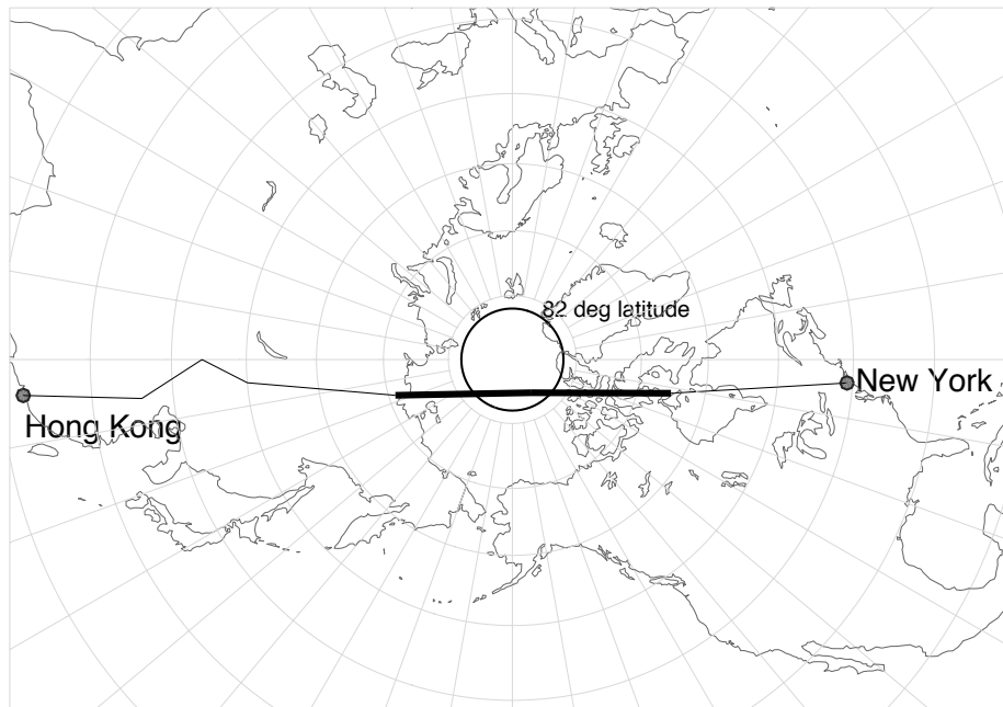
Figure 1. Example trans-polar route from New York to Hong Kong via Polar 3. The bold line indicates where communication is out of range of the VHF infrastructure and is only possible via HF links.
