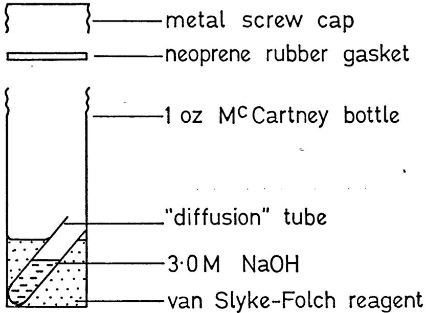
B. Combustion-diffusion vessel-wet samples
