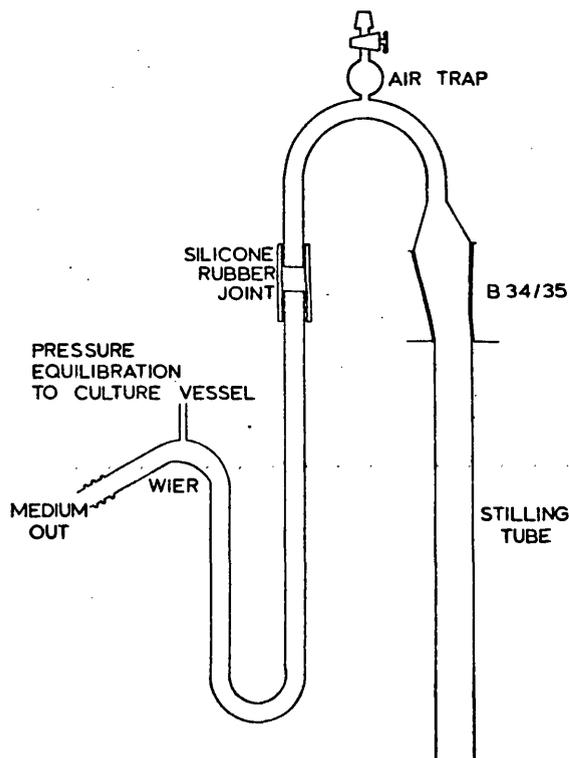
FIG. 17. Siphon tube unit.
