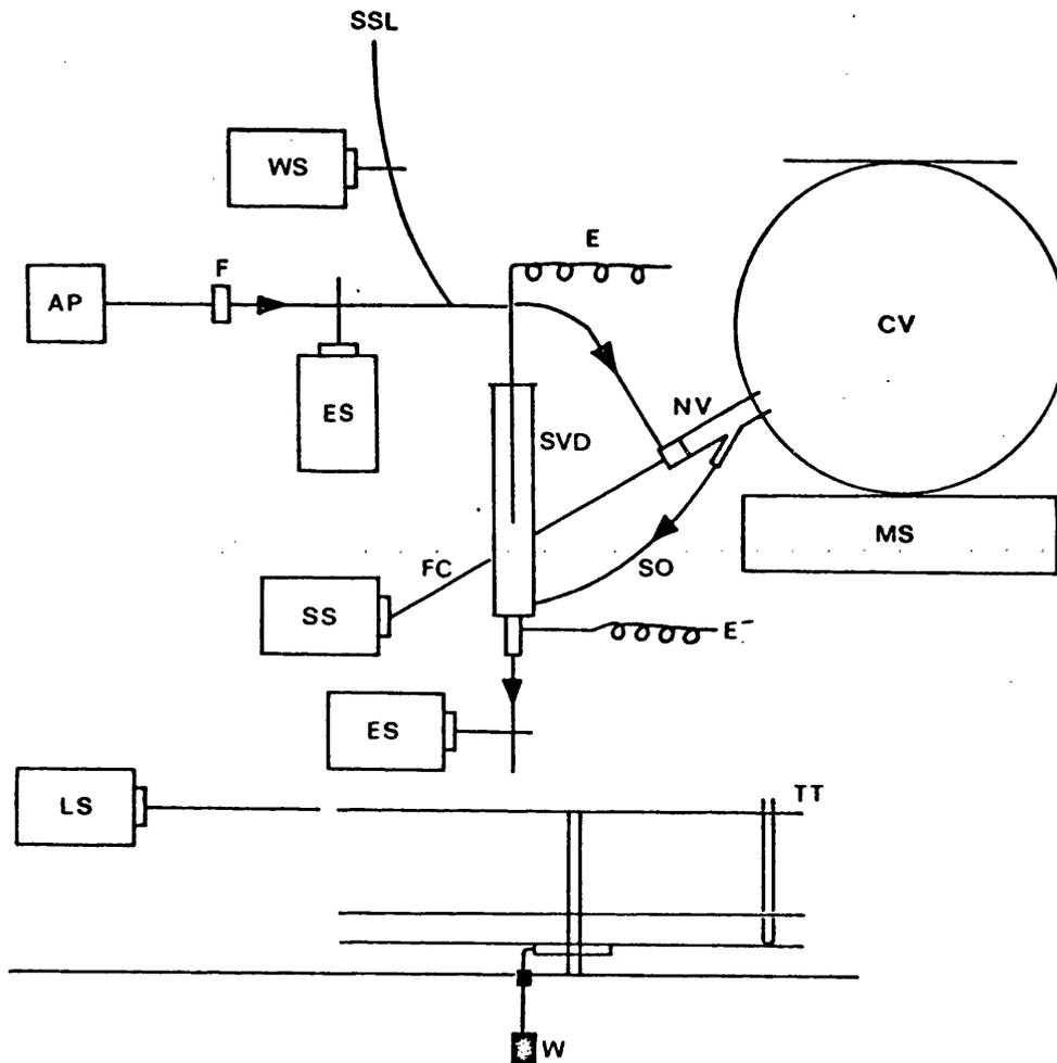
FIG. 13. Flow diagram showing operation of the automatic sampling assembly.
