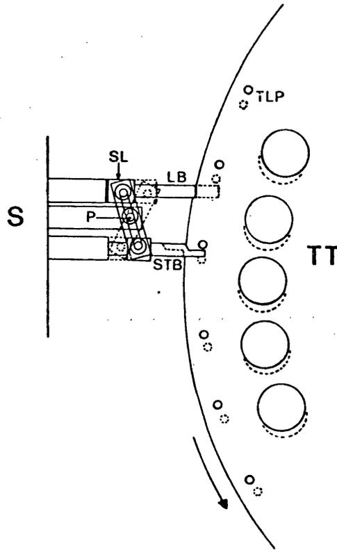
FIG. 14. Turntable and latching device. Direction of rotation of turntable indicated by arrow. Rest position of latching device shown as solid line, energized position as broken line.
