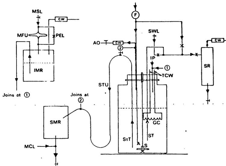
FIG. 16. Flow diagram for closed continuous culture system. Conventions and key as Fig. 11 with the following additions:
