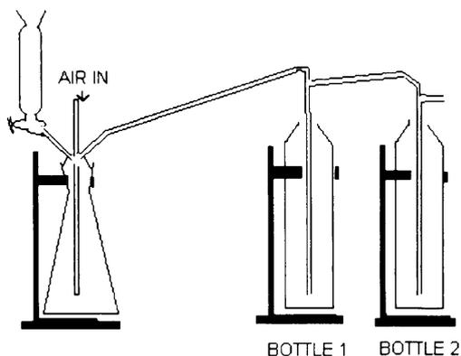
15mL of 0.025 mol/L iodine solution were pipetted into bottle 1, followed by a little (1 or 2mL) dilute hydrochloric acid. A few drops of starch indicator were added and the solution was titrated with 0.05 mol/L sodium thiosulphate solution.
