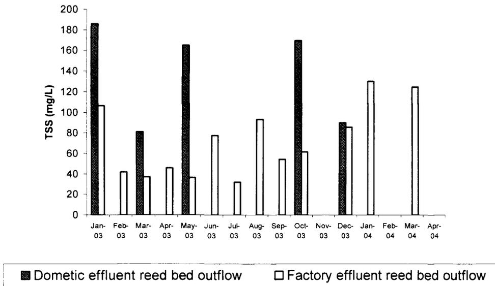
Figures 6.9a to 6.9d show that there was a considerable difference in the quality of the outflow effluent from the domestic and factory effluent reed bed systems. However the results presented in this way do not make clear how the development and modification of the reed bed system over time effected treatment performance.
