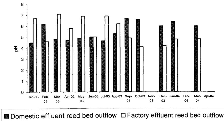
The explanation for the apparent reversal in effluent treatment performance from the two reed bed systems in some of the months was that the type of effluent loaded onto the reed beds was reversed. The domestic effluent reed beds were loaded with factory effluent and the factory effluent reed beds were loaded with domestic effluent to try to encourage reed growth on the factory effluent reed beds.
