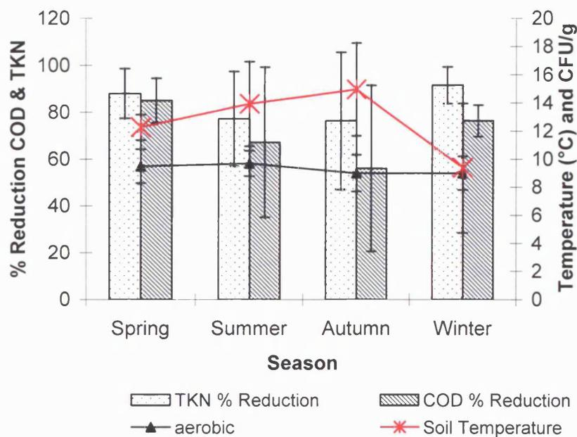
Figure 4.1 shows seasonal treatment performance averages which were calculated using all available loading period data. The results show that soil temperatures were lowest in winter (9.4°C). Soil temperatures increased through spring and summer and were highest in autumn (15.0°C). Lower COD reduction occurred in summer and autumn than in spring and winter. Greatest COD reduction occurred in spring (85%). Greater
