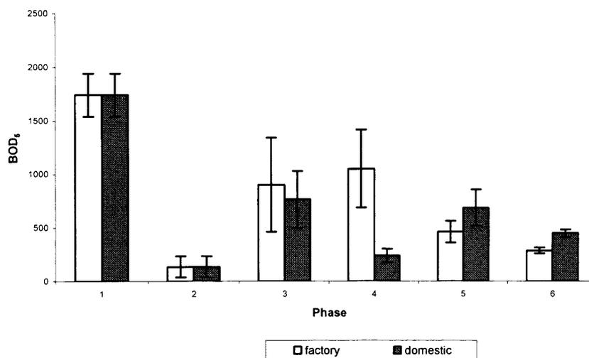
The outflow BOD<sub>5</sub> from the factory effluent reed beds was compared between *Phase 1* and *Phase 3*; *Phase 1* and *Phase 4*; *Phase 1* and *Phase 5*; and *Phase 1* and *Phase 6*. It
