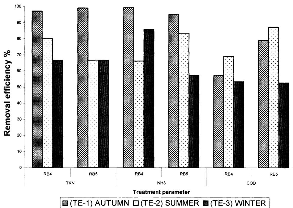
Figure 5.2 shows that COD reduction was most efficient in both reed beds 4 (69%) and 5 (87%) in the summer (TE-2). COD reduction under winter weather conditions was less effective (TE-3) than in summer.
