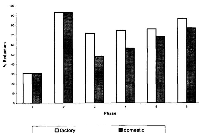
Phase: 1 = stabilisation pond, 2=combined, 3=separate, 4=switched, 5=combined, 6=separate
