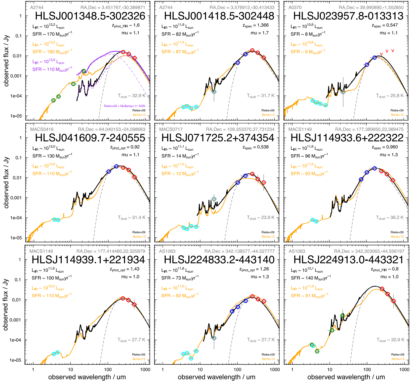
Figure 7. Example IR SEDs illustrating the observed photometry and fits. In each panel, observed (uncorrected) fluxes are shown by open circles: IRAC=cyan, MIPS=grey, WISE =green, PACS=blue, SPIRE=red. Non-detections ( 5\sigma upper limits) are denoted by a ‘v’. Also plotted are the best-fitting modified-blackbody (grey dashes), Rieke et al. (2009) template (black solid line) and Berta et al. (2013) template (orange solid line). Derived IR properties from each of the two template sets (in matching colours) take into account the magnification, \mu (shown to the right). Redshifts are spectroscopic ( z_{\text{spec}} ), optical photometric ( z_{\text{phot, opt}} ) or IR-derived ( z_{\text{phot, FIR}} ; see Section 4.4.1). For SEDs with a fitted AGN component, the two component model and star formation IR properties are shown in purple.
