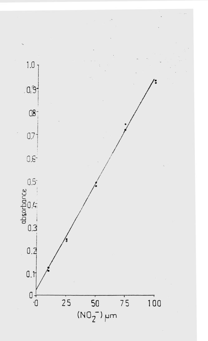
Fig. 2.4 Calibration curve: Absorbance of potassium nitrite standard solutions (2 ml) plus nitrite assay mixture (see text) after 10 minutes incubation, versus nitrite concentration. Absorbance measured at 545 nm. Curve = line of best fit after linear regression (n = 2). Equation: Absorbance = 0.094 (nitrite concentration) + 0.083
