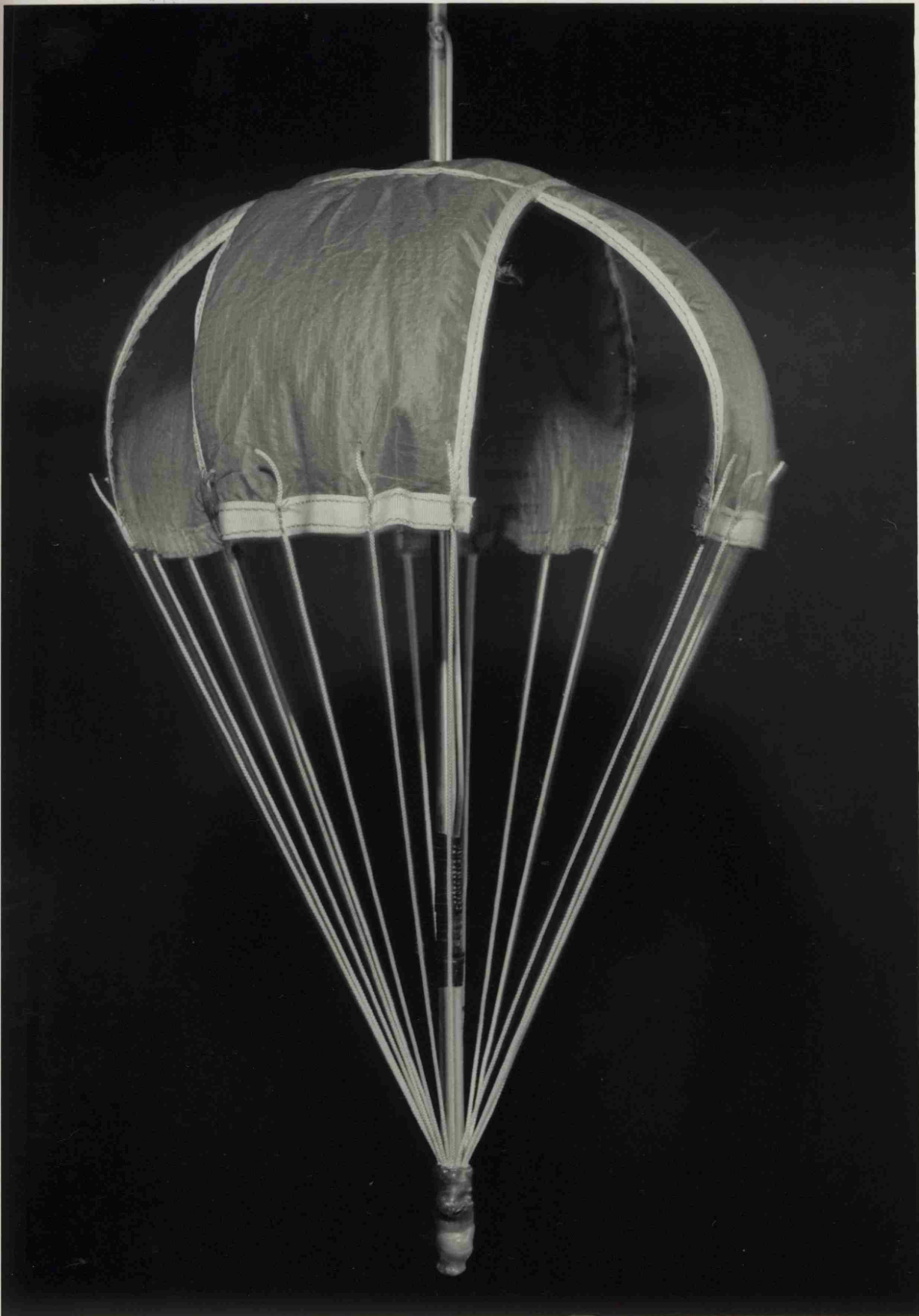
Figure 4.7 cruciform parachute, with arm ratio of 4:1.
