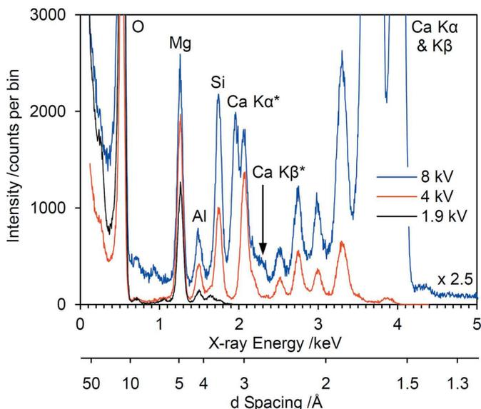
**Figure 3** Back-reflection spectra of limestone A at three different excitation voltages/emission currents: 8.0 kV/0.1 mA, 4.0 kV/1.0 mA for Ca *K* suppression, and 1.9 kV/2.0 mA for Si *K* suppression (cf. Fig. 1). The 8.0 kV data have been multiplied by 2.5 to allow easier comparison. The Si *K* suppression data are taken from the whole imaging area of the CCD rather than the top third only because of the relatively low intensity.
