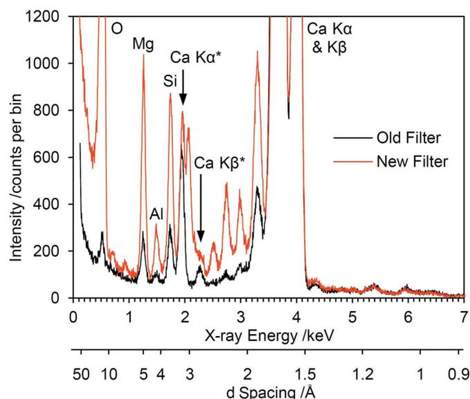
**Figure 2** Back-reflection spectra of limestone A with the two different optical filters (see text for details). The excitation voltage is 8.0 kV in each case, and the emission currents are 0.4 mA for the ‘old’ filter and 0.1 mA for the ‘new’ filter. The fluorescence peaks are labelled, escape peaks with an asterisk; the unlabelled peaks are due to diffraction, including the weak features above 4 keV.
